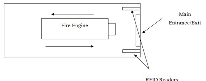
Figure 2: RFID System for Fire Service
