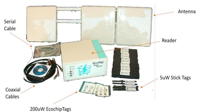
Figure 1: Trolley Scan RFID-Radar System <sup>3</sup>
