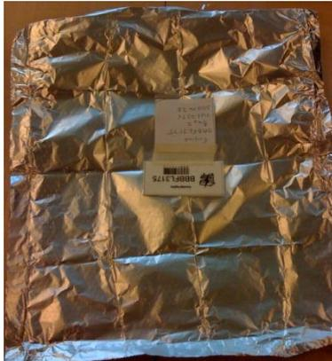
**Figure 9: Test 16: Passive Tag on Foil**
