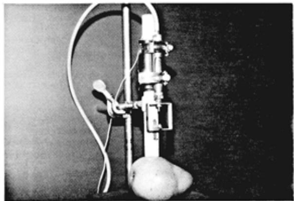
Figure 1: A photograph of the impact probe with the impact mass in the return position
