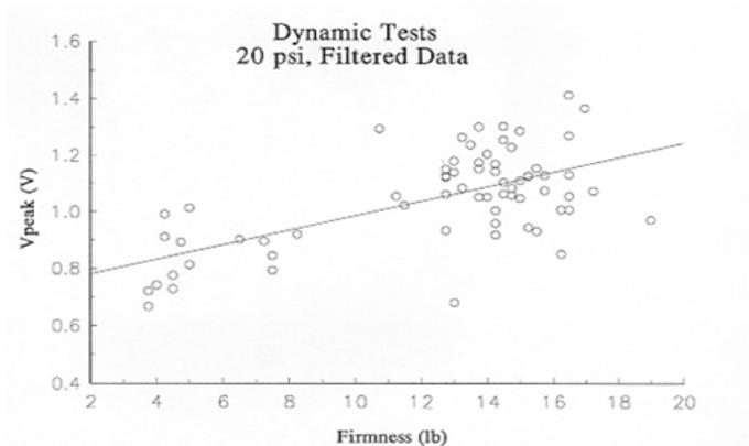
Figure 3: A Impact tests to pears moving through handling system with air pressure 20 psi
