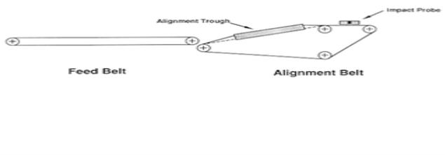
Figure 2: A side-view of the prototype handling system, with fruit flow from left to right
