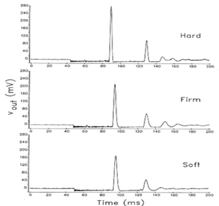
Figure 3: b Impact probe out put for hard ( $f=84.5N$ ) firm ( $f=50.0N$ ) and soft ( $f=13.3$ ) pears
