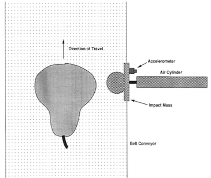
Figure 5: A top –view of the modified impact probe mounted on a belt conveyor
