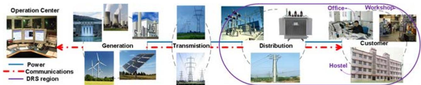
Figure 1: An example of a smart grid with DRS
