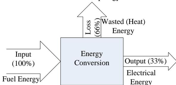
Figure 2: Fuel energy conversion of the conventional electricity grid
