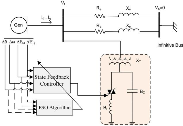
Fig. 1. Single machine-infinite bus system model with SVC.
