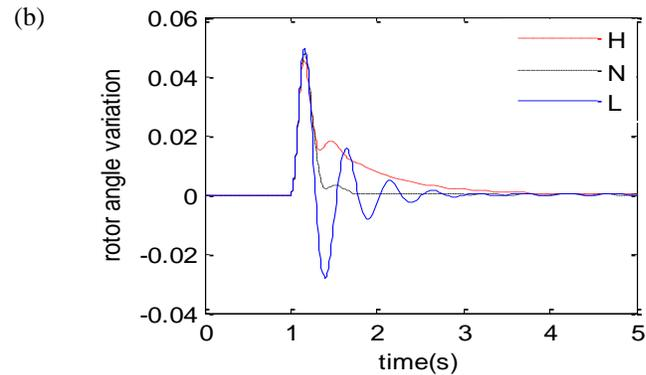
Fig. 8. System Dynamic Response for Six Cycles Fault Disturbance With Normal, Light and Heavy Loading. (A) Rotor Speed Variation, (B) Rotor Angle Variation.
