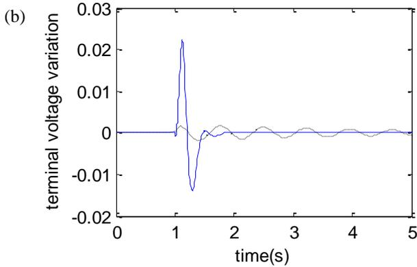
Fig. 6: System Dynamic Response for Six Cycles Fault Disturbance. (a) Internal Voltage Variation, (b) Terminal Voltage Variation, Solid (SVC based Controller), Dash (without Controller)
