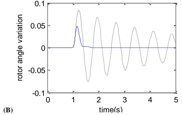
Fig. 7. System Dynamic Response For Six Cycles Fault Disturbance. (A) Rotor Speed Variation, (B) Rotor Angle Variation, Solid (SVC Based Controller), Dash (Without Controller)
