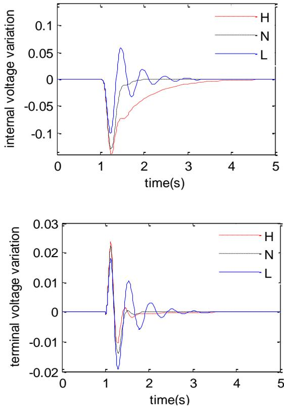
Fig. 9. System Dynamic Response for Six Cycles Fault Disturbance with Normal, Light and Heavy Loading. (A) Internal Voltage Variation, (B) Terminal Voltage Variation
