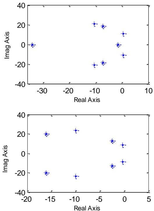
Fig. 11: Eigenvalue Distribution of the System. (a) Heavy Loading, (b) Light Loading. (\* with Controller, + without Controller)
