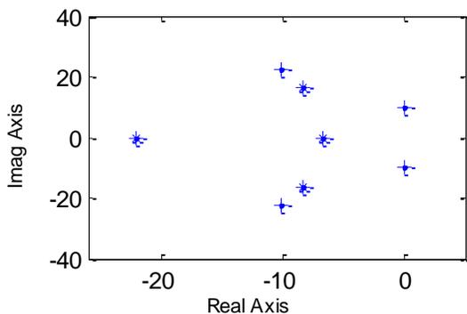
Fig. 10: Eigenvalue Distribution of the System in case of Normal Loading. (\* with Controller, + without Controller)
