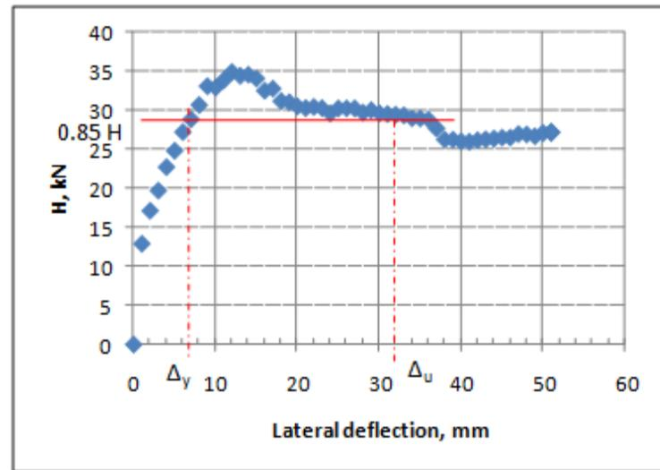
Figure 10: Definition of Frame Ductility [4]
