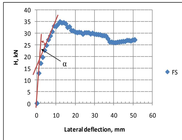
Figure 4: Fully Infilled Frame Behaviour under Lateral Loading
