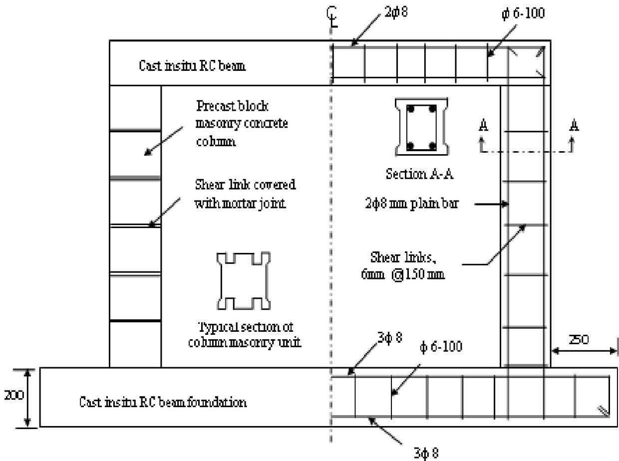
Figure 2. Hybrid RC Frame Details
