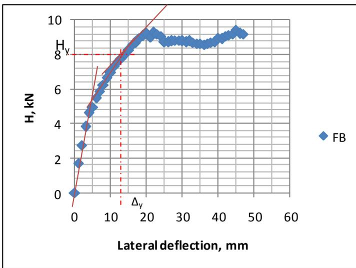
Figure 11: Definition of Frame Stiffness [4]
