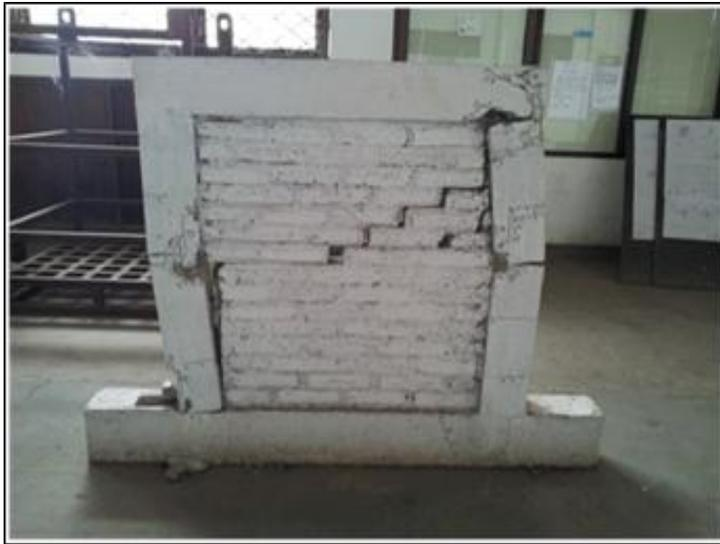
Figure 5. Failure pattern on hybrid frame with fully infill wall
