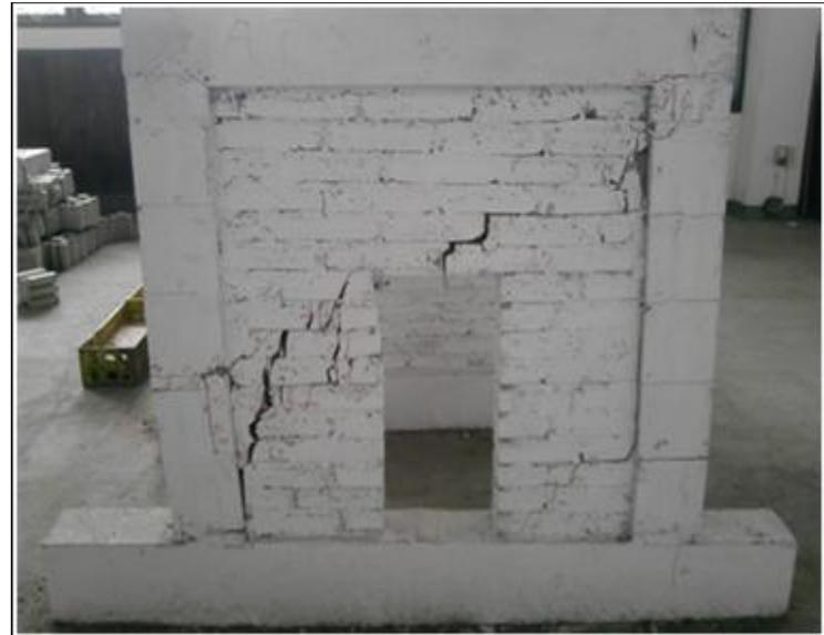
Figure 7: Failure pattern of FDC Hybrid Frame under Lateral Loading
