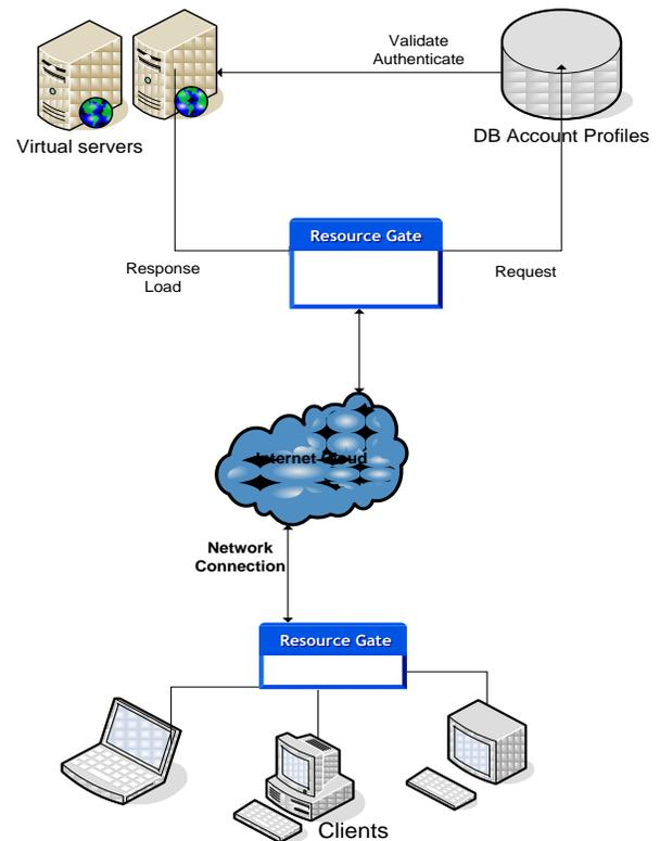
Figure 4: System overview of ResourceGate
