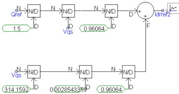
Fig. 6 Reactive power control scheme: primary stage
