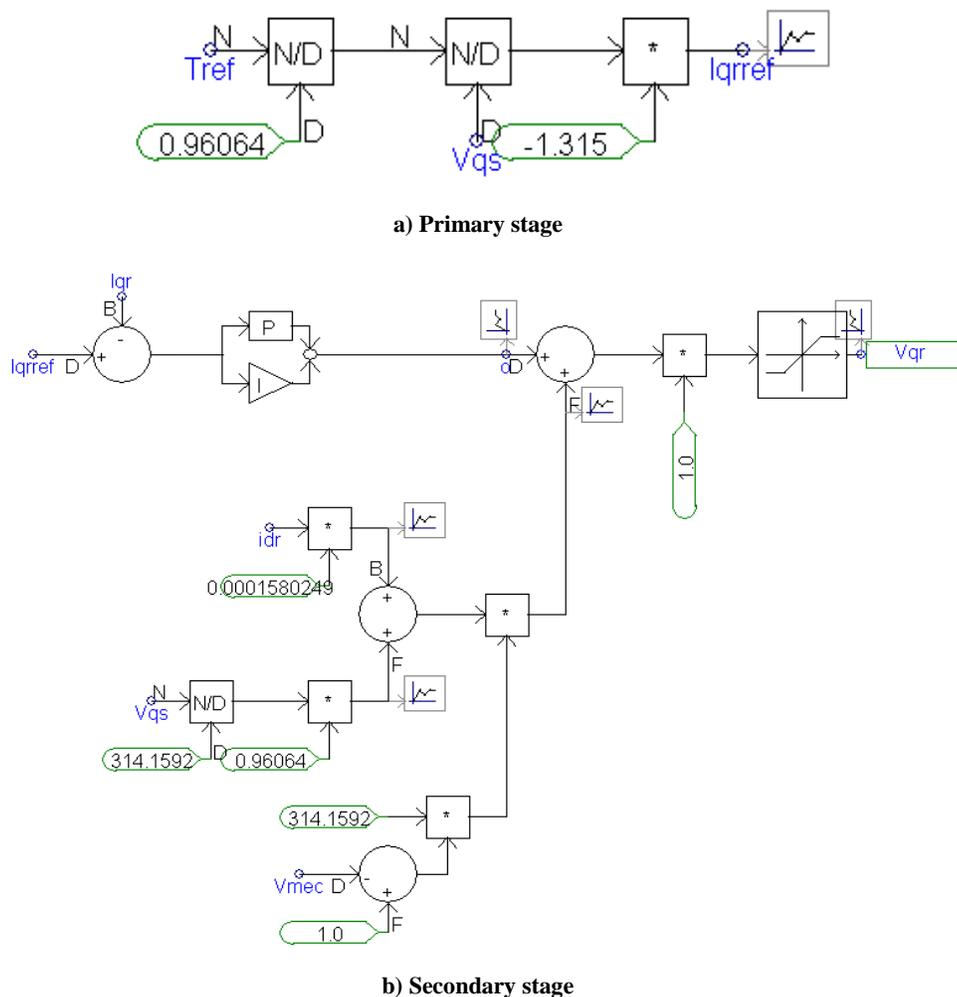
Fig. 4 Speed control scheme based on vector control
