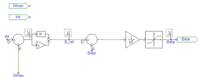
Fig. 2 Pitch angle control block diagram
