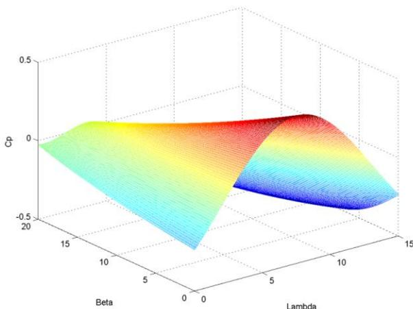
Fig. 1 Typical  $C_p$  versus TSR
