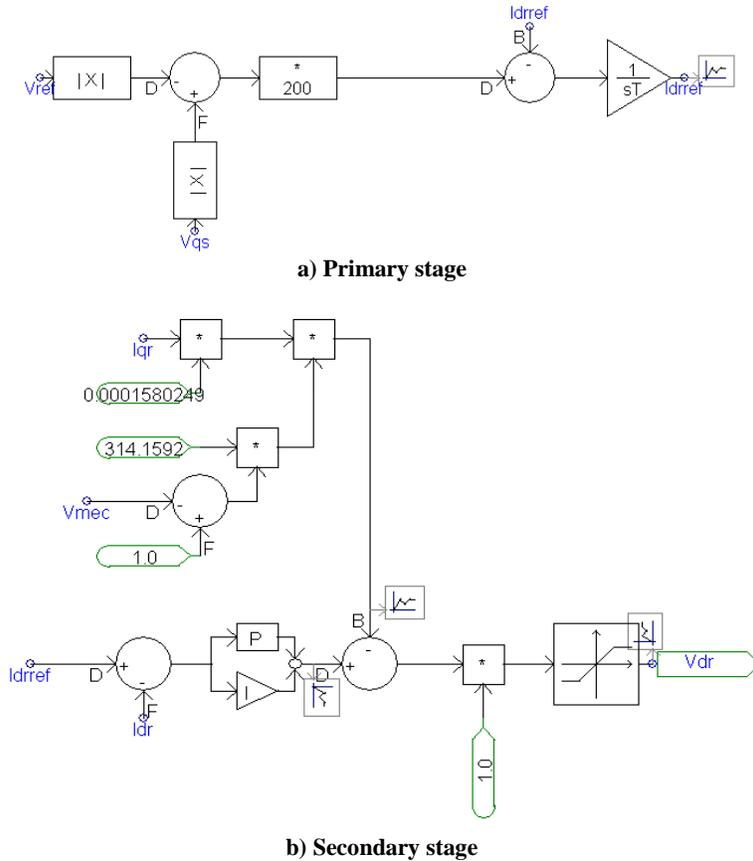
Fig. 5 Voltage control scheme based on vector control
