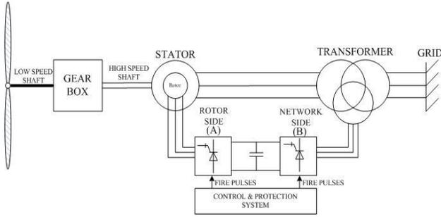
**Fig.3 DFIG overall system in a wind turbine-generator**
