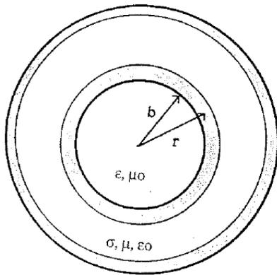
Figure 3: Outer Conductor geometry
