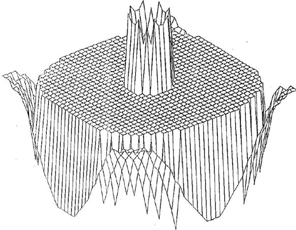
Figure 1: 3D Representation of the skin effect in a coax cable
