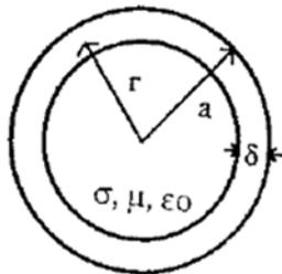
Figure 2: Inner Conductor geometry
