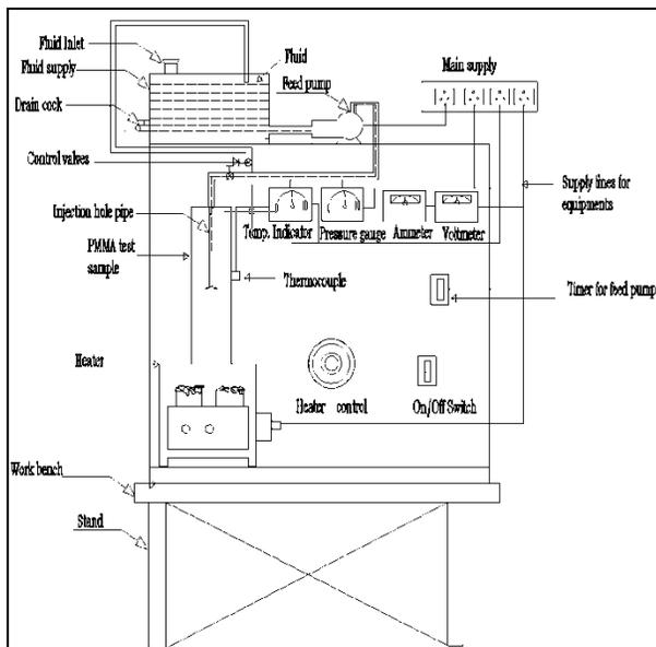
Fig.1. Experimental set up for Hydrofracturing process
