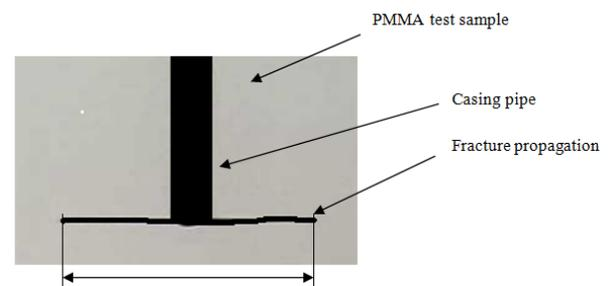
Fig-2 shows the highest Fracture length of 580mm was observed at a pressure 7 N/mm<sup>2</sup>, Temperature of 55°C and
