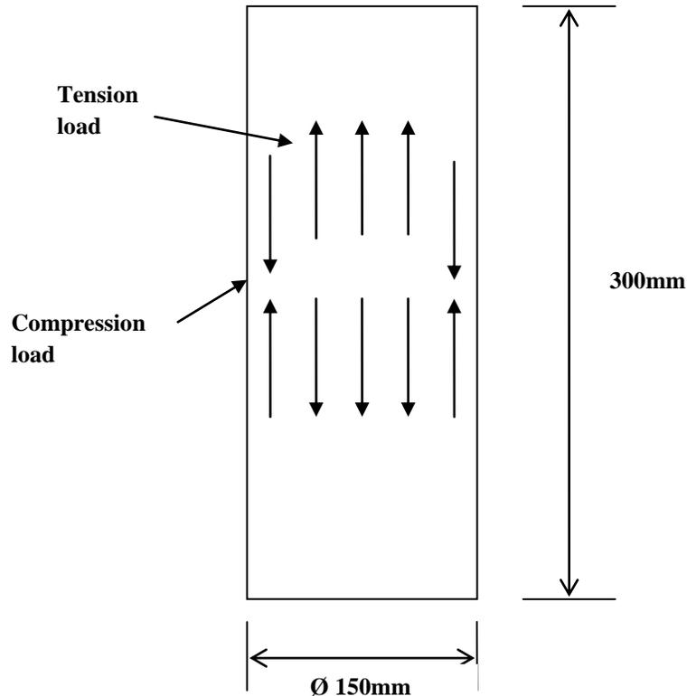
Fig-3 shows the PMMA sample with dimensions and load acting due to temperature effect
