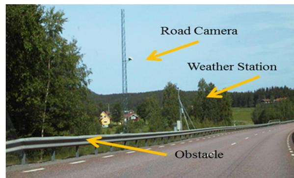
Figure 8.1 Typical obstacles around a weather station located with road 83 in Gävleborg county, Sweden (Source: STA)
