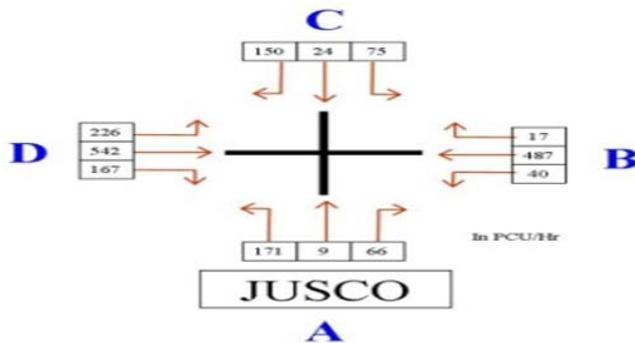
Figure 3. Traffic Flow at Jalan Perdagangan Intersection (read in conjunction with figure 2)
