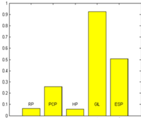
Figure 2 .Artificial lift result for the oil field by TOPSIS model
