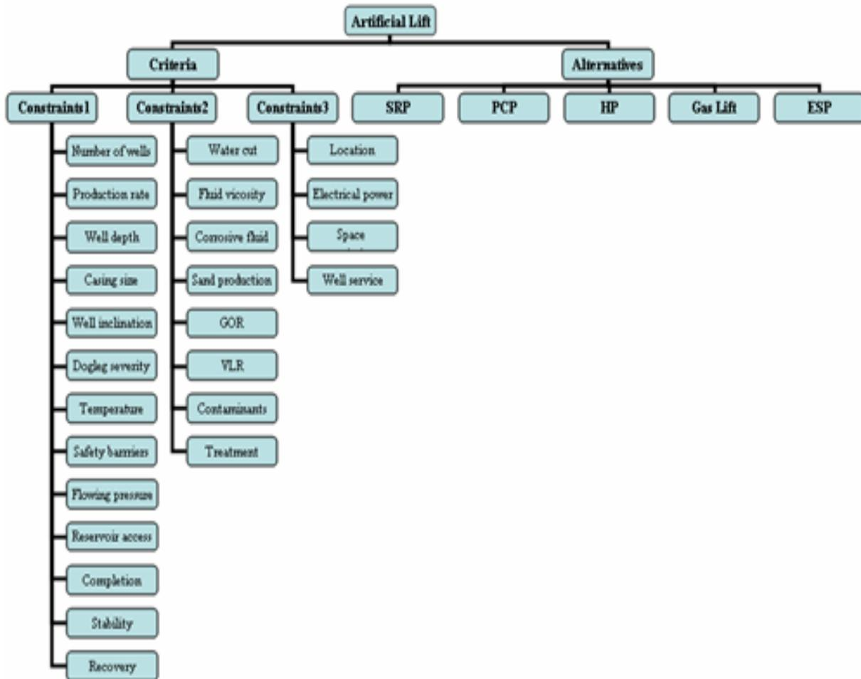
Figure 1. The Alternatives and criteria for artificial lift selection
