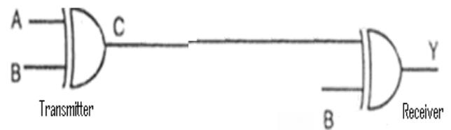
Figure 1.2. Encryption and decryption by using same key
