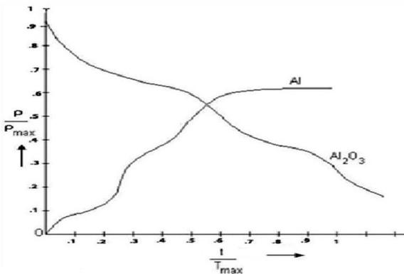
Fig.2: Resistivity variation of Al, and Al<sub>2</sub>O<sub>3</sub> with temperature
