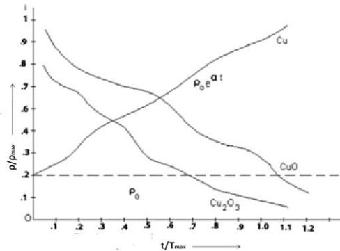
Fig.1: Variation of Resistivity of Cu, CuO and Cu<sub>2</sub>O<sub>3</sub>
