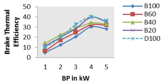
Fig. 5 Variation of bte with concentration of mahua at different loads
