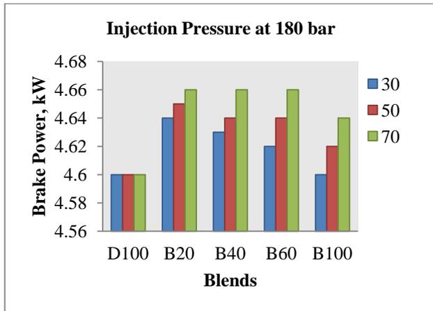
Fig. 3(a) Effect of fuel temperature on power output for blends at injection pressure of 180 bar
