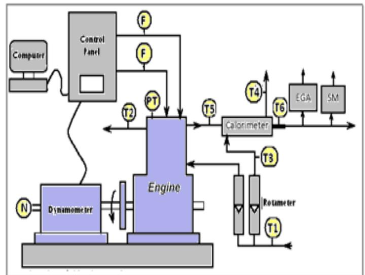
**Fig 1: Experimental Test Rig.**
