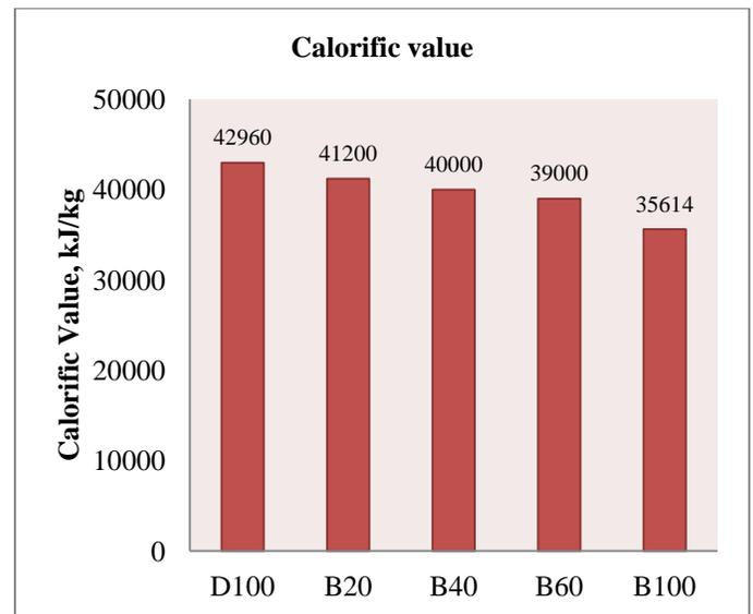
Fig. 2(c) Variation of calorific value with concentration of mahua
