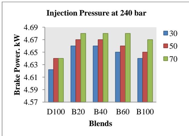
Fig. 3(b) Effect of fuel temperature on power output for blends at injection pressure of 240 bar
