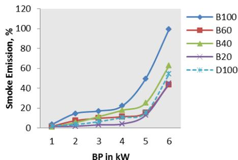
Fig. 6 Variation of smoke emissions with concentration of mahua at different loads
