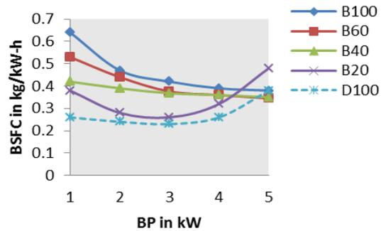
Fig. 4 Variation of BSFC with concentration of mahua at different loads
