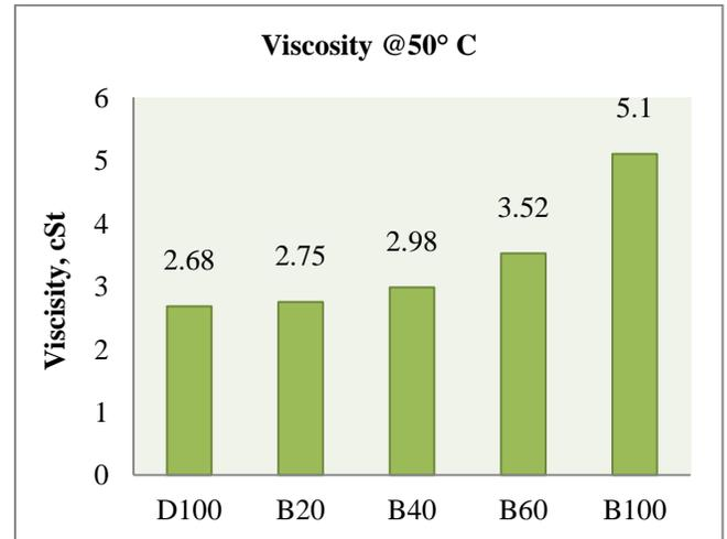
Fig. 2(b) Variation of viscosity with concentration of mahua
