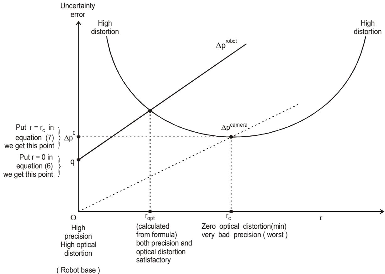
Fig. 2 : To determine the optimal position for the placement of the workspace fixture in the workspace of robot
