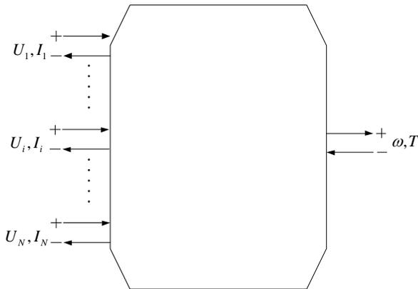
**Figure 1: An electromagnetic system with N electrical ports and one mechanical port electromagnetic**
