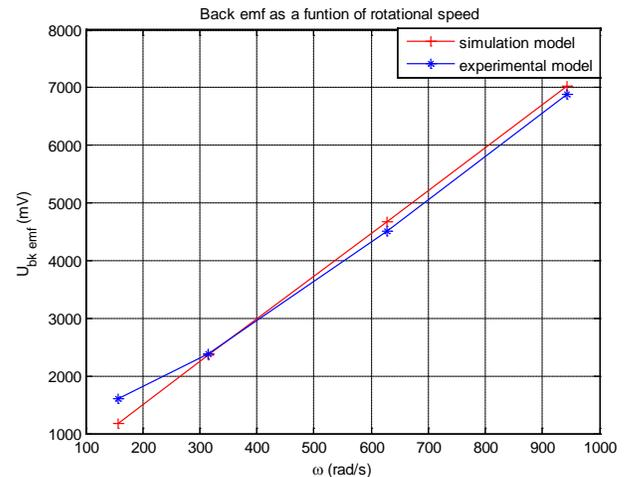
Figure 6: Back emf comparison of experimental and simulated models against rotational speed
