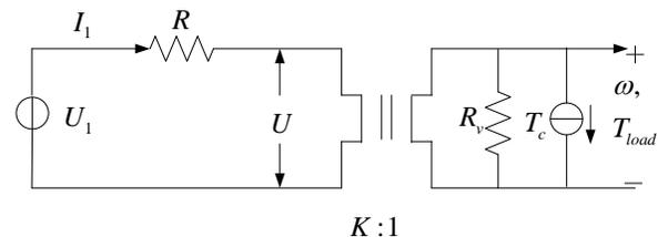
Figure 4: Circuit-diagram of motor an improved figure 3
