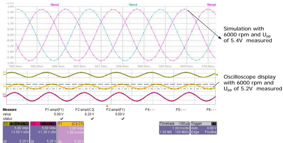
Figure 9: Back emf view of simulation and oscilloscope with 6000rpm speed
