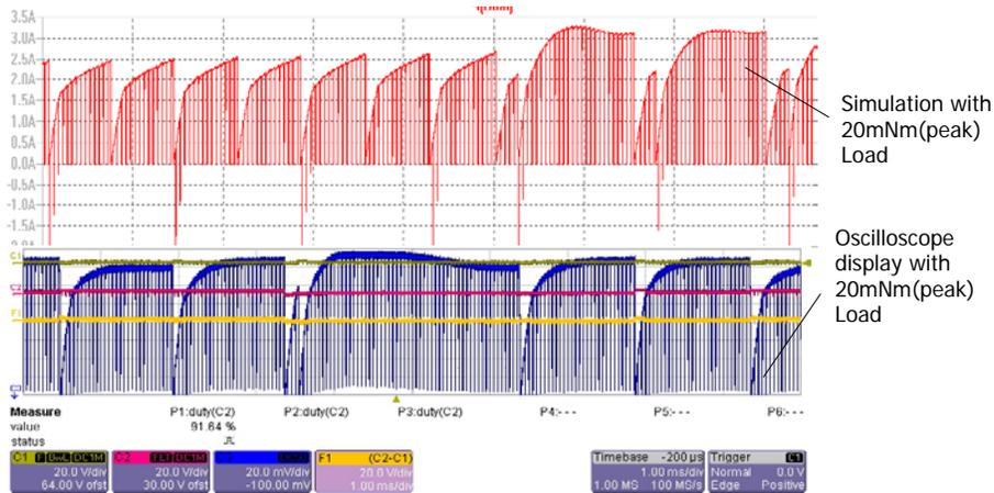
Figure 8: Current view of simulation and oscilloscope at 20mNm (peak) Load
