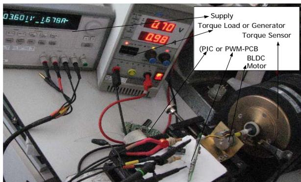
Figure 5: Measurement set-ups with Torque sensing machine to determine BLDC motor behaviour
