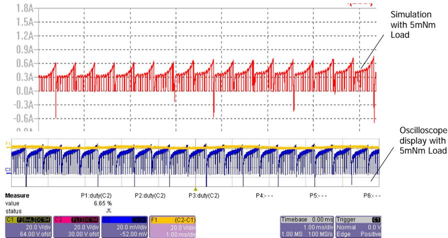
Figure 7: Current view of simulation and oscilloscope with Toque load 5mNm
