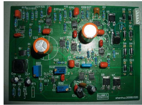
Fig. 11: PCB prototype of a self-powered energy harvesting circuit based on ESSH technique [54]
