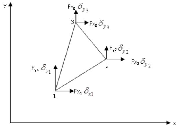
Figure 1: Two dimensional triangular element typical of that used in plane stress problems.
