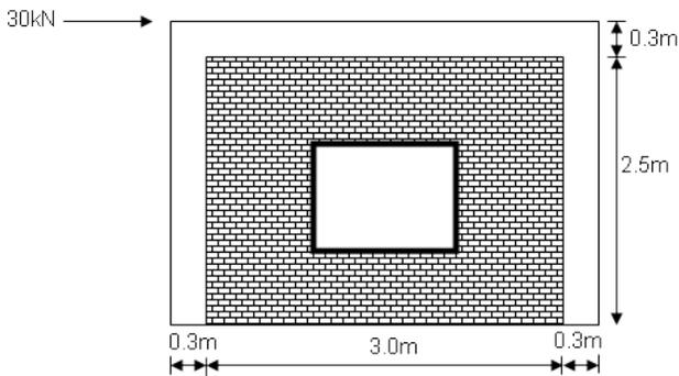
**Figure 3: Infilled reinforced concrete frame structure with central opening**
