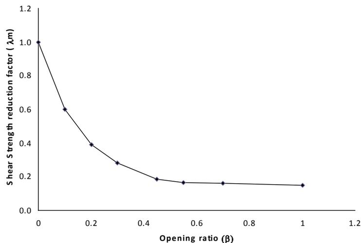
Figure 6: Variation of shear strength reduction factor of infilled frame with opening ratio for a case of central opening.
