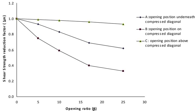
Figure 7: Variation of shear strength reduction factor  $\lambda_m$  of infilled frame with opening ratio for different position of opening.
