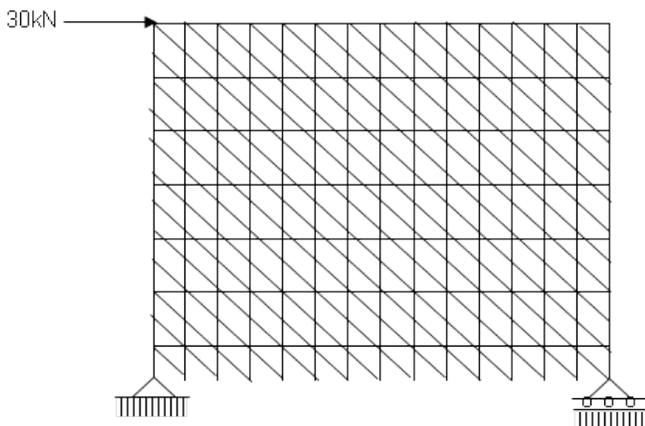
**Figure 4: Triangularly meshed micro-model ready for finite element analysis**
