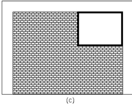
Figure 5: Different configuration of opening position on an infilled frame structure
