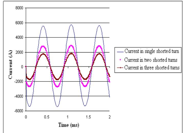
**Figure 7: Currents in different number of short circuited turns.**
