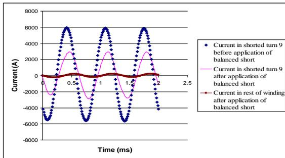
Fig.11. Single faulty turn predicted currents before and after application of balanced short.
