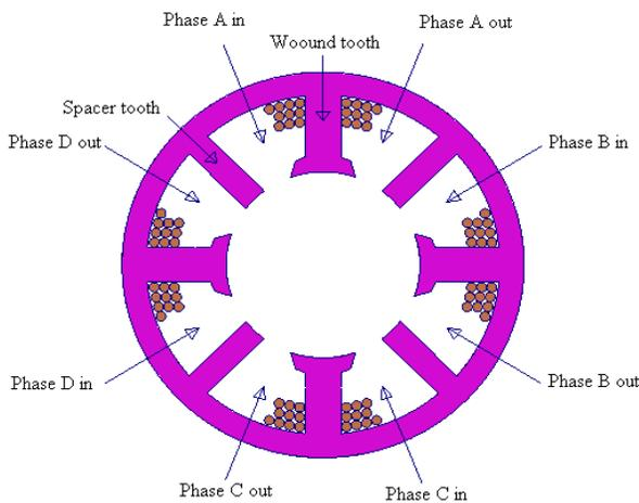
Figure 1: Stator 2DFE model of the 120kW machine.
