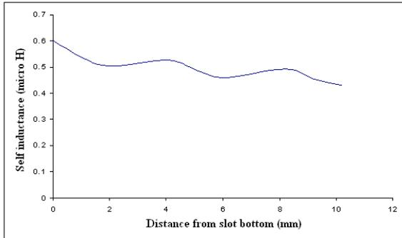
Figure 3: Variation of self-inductance of turn versus its position
