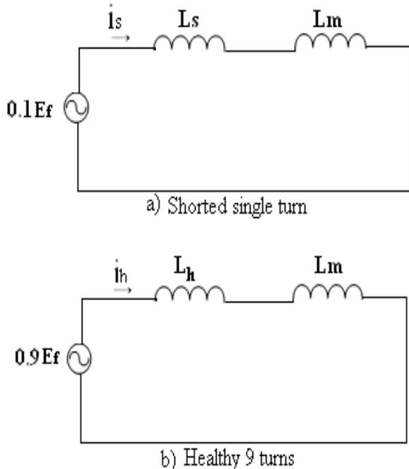
Figure 8: Equivalent circuits after application of balanced short
