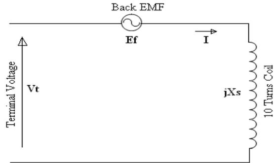
Figure 5: Equivalent circuit per phase
