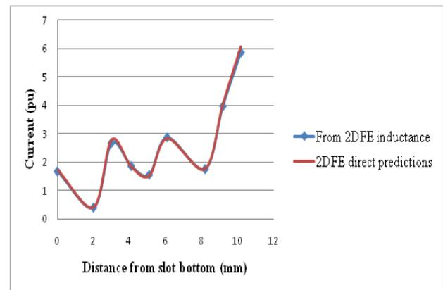
**Figure 9: Variation of current in single faulty turn after applying balanced short**
