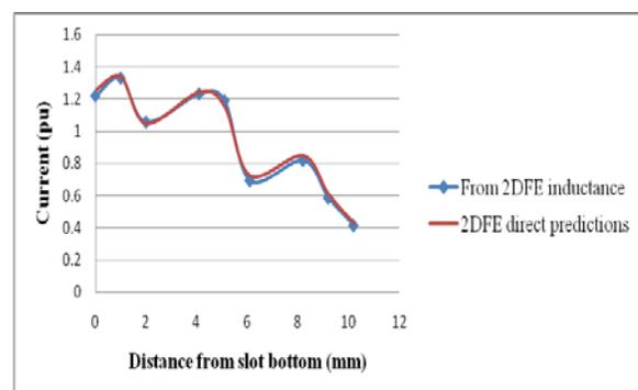
**Figure 10: Variation of current in healthy turns after applying balanced short.**
