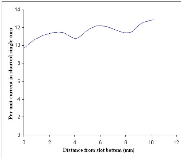
**Figure 6: Variation of Current in Shorted Turn versus its position**
