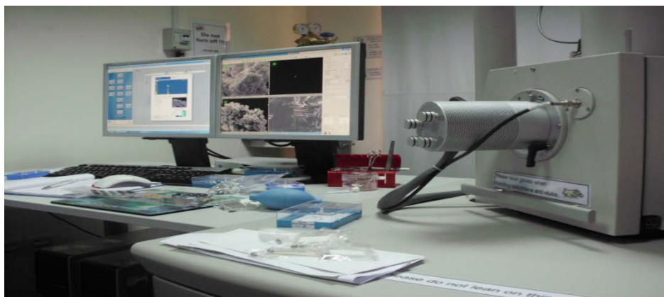
Figure 5: Scanning Electron Microscope – The Petroleum Institute (Philips-FEI Quanta 200)
