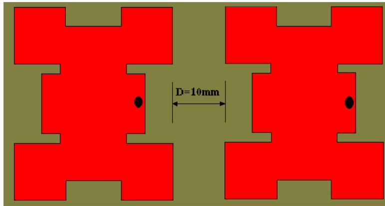
Fig 3. A 2x 2 MIMO systems using the proposed antenna
