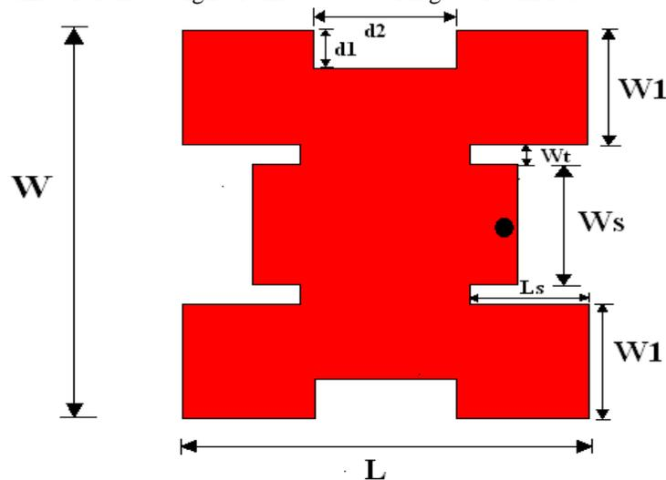
Fig.1 Modified Back to Back E shape patch antenna
