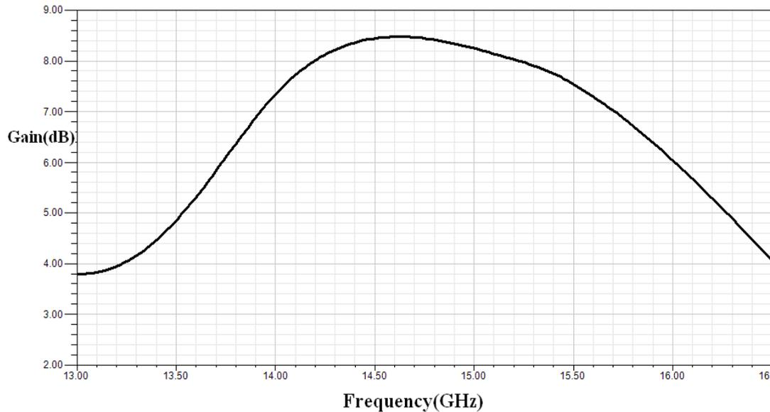
Fig.7 Gain plot of the 2x2 MIMO System
