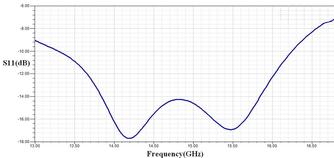
Fig 2. Return loss of the proposed antenna
