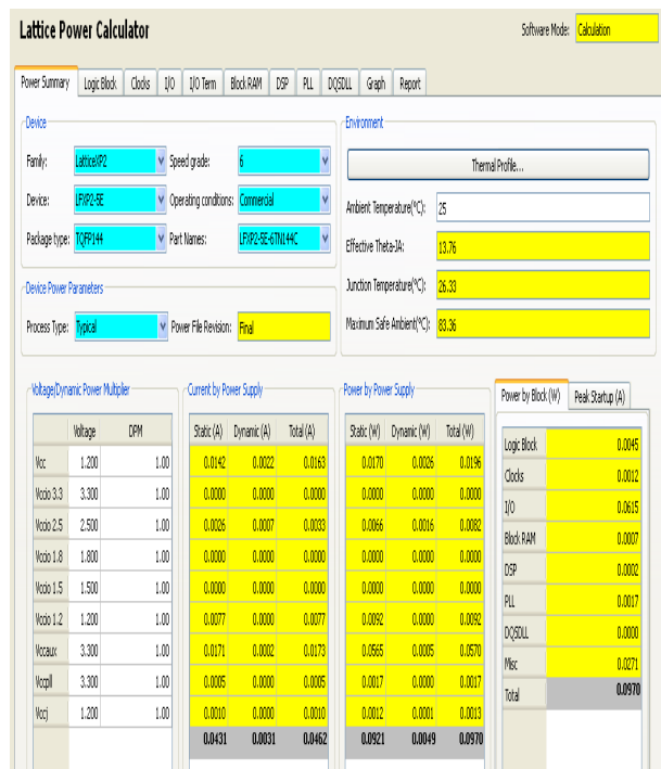
Fig. 4. Power calculation of with gated clock module at 50 MHz clock
