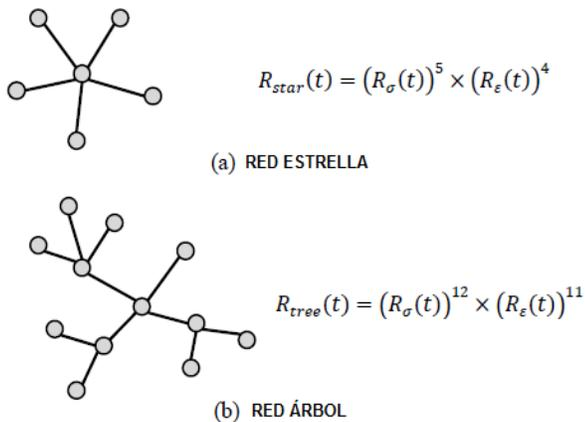
Figure N° 4. Types of networks using block diagrams. [21]
