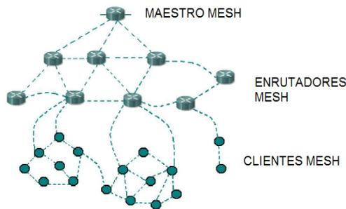
Fig. No 1. Mixed in Mesh Architecture
