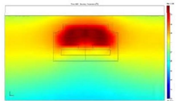
**Fig. 11. Temperature field in the soil around the buried landmine 3600s after heating phase. The thermal diffusion process has already taken place and the temperature of the free soil and over the buried landmine tends to become uniform.**
