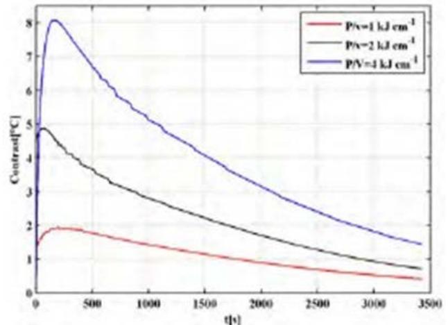
Fig. 12. Contrast function for different  $P/v$  ratio. Increasing the  $P/v$  ratio, the temperature contrast increases.
