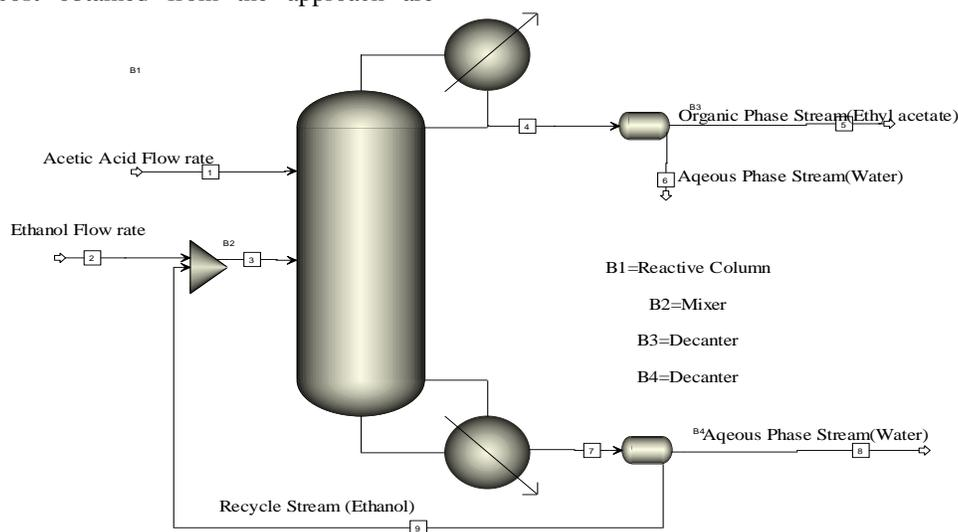
Fig. 1: Process flow diagram (PFD) for the optimal design
