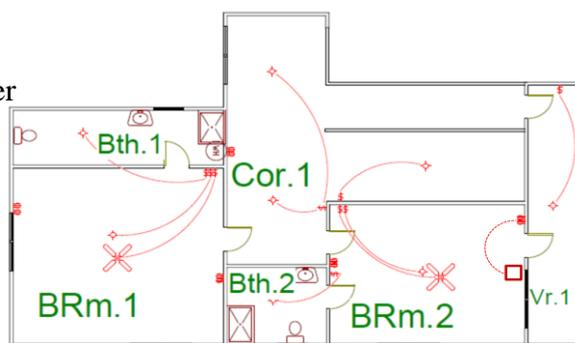
Figure 3: Electrical Plan of First Floor
