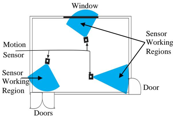
Figure 5: Plan of Room Showing Motion Sensor Position and Active Working Region for the Intruder Alert System
