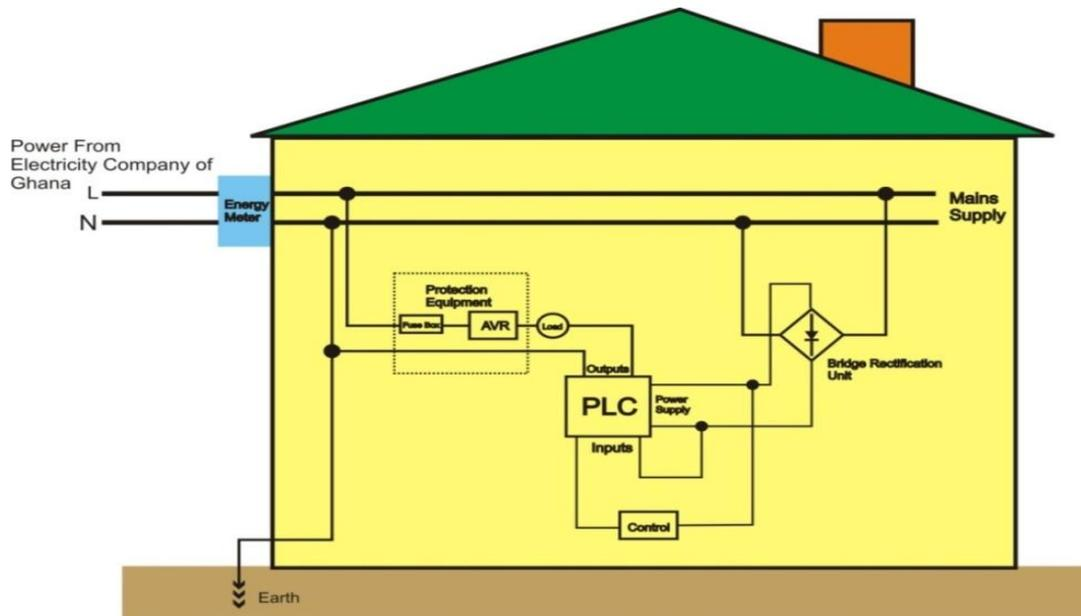
Figure 1: Basic Connections of the PLC System Integrated into the Home
