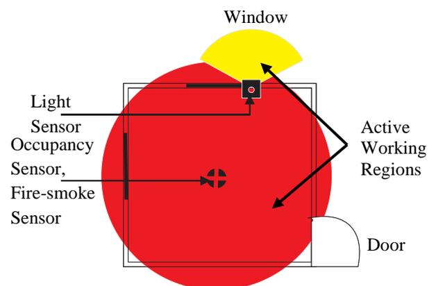
Figure 4 Plan of Room Showing Occupancy, Fire-smoke and Light Sensor Positions and Catchment Areas.
