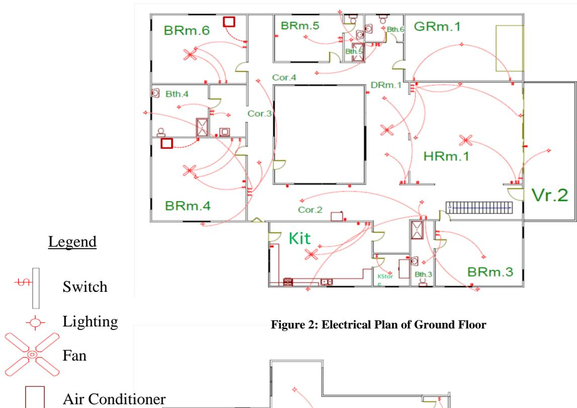
Figure 2: Electrical Plan of Ground Floor
