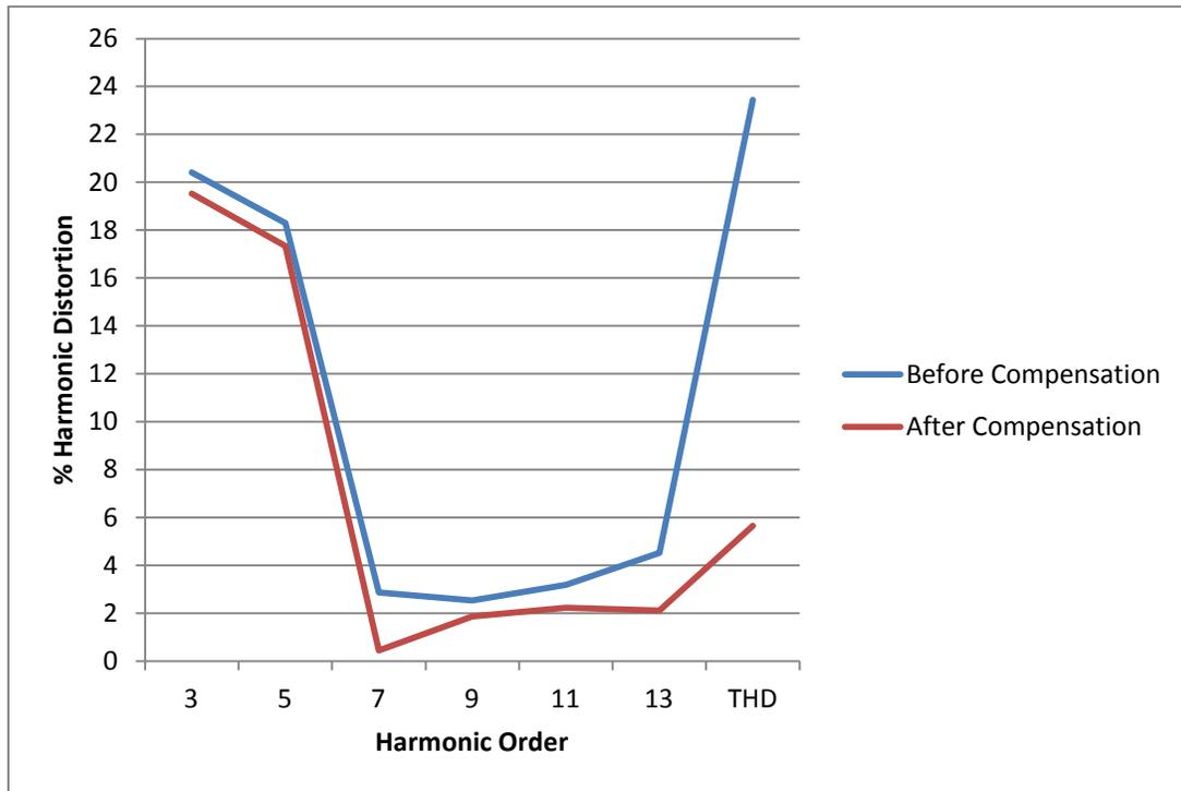
Fig. 12: Harmonic Distortion for Second Experiment of 7<sup>th</sup> Harmonic Tuned Filter at 348 Hz
