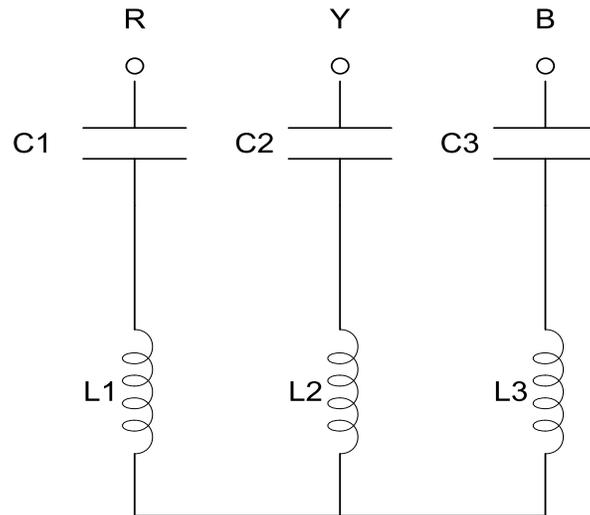
Fig. 3: Shunt Passive Filter
