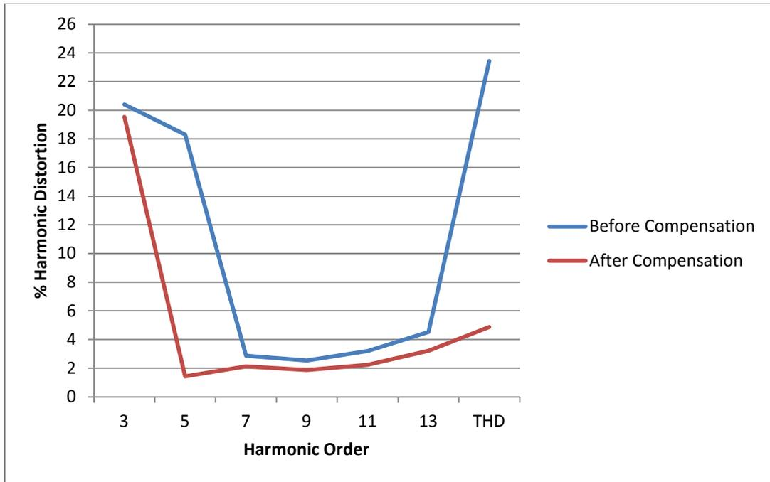
Fig. 8: Harmonic Distortion for the Second Experiment of 5<sup>th</sup> Harmonic Tuned Filter at 256 Hz
