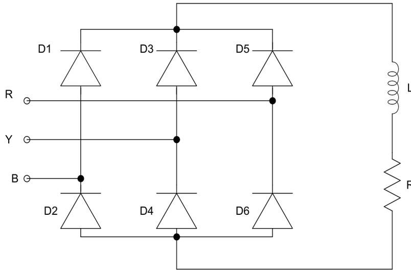
Fig. 2: Non-linear Load
