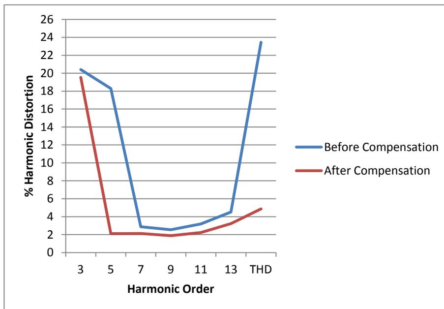
Fig. 7: Harmonic Distortion for the First Experiment of 5<sup>th</sup> Harmonic Tuned Filter at 252 Hz
