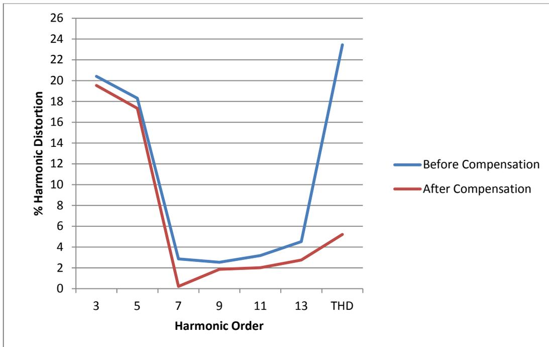
Fig. 10: Harmonic Distortion for the First Experiment of 7<sup>th</sup> Harmonic Tuned Filter at 356 Hz
