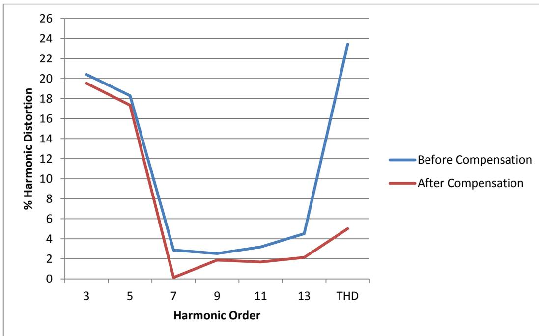
Fig. 11: Harmonic Distortion for the Second Experiment of 7<sup>th</sup> Harmonic Tuned Filter at 364 Hz
