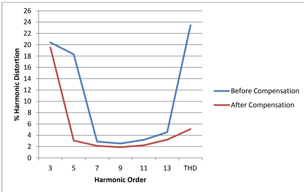
Fig. 9: Harmonic Distortion for the Third Experiment of 5<sup>th</sup> Harmonic Tuned Filter at 247 Hz
