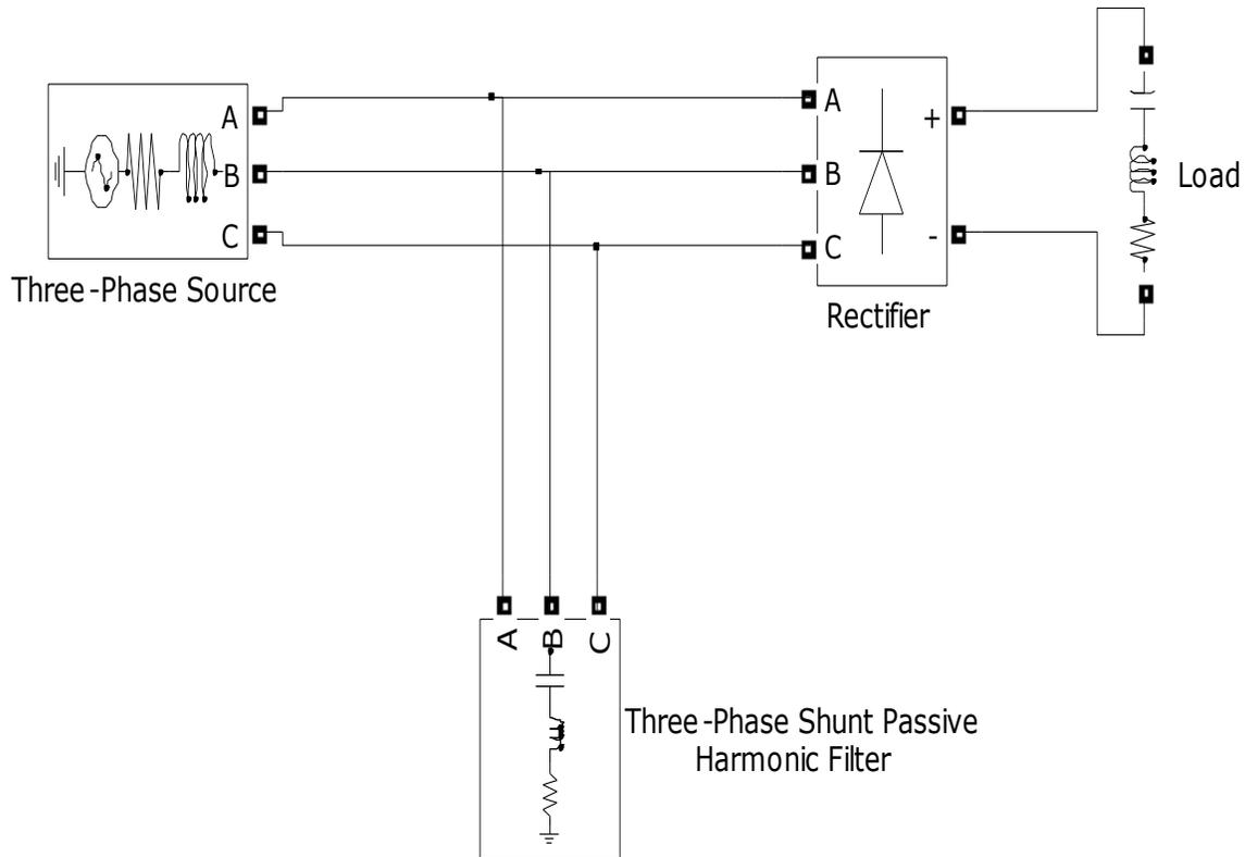
Fig. 5: Simulation Diagram
