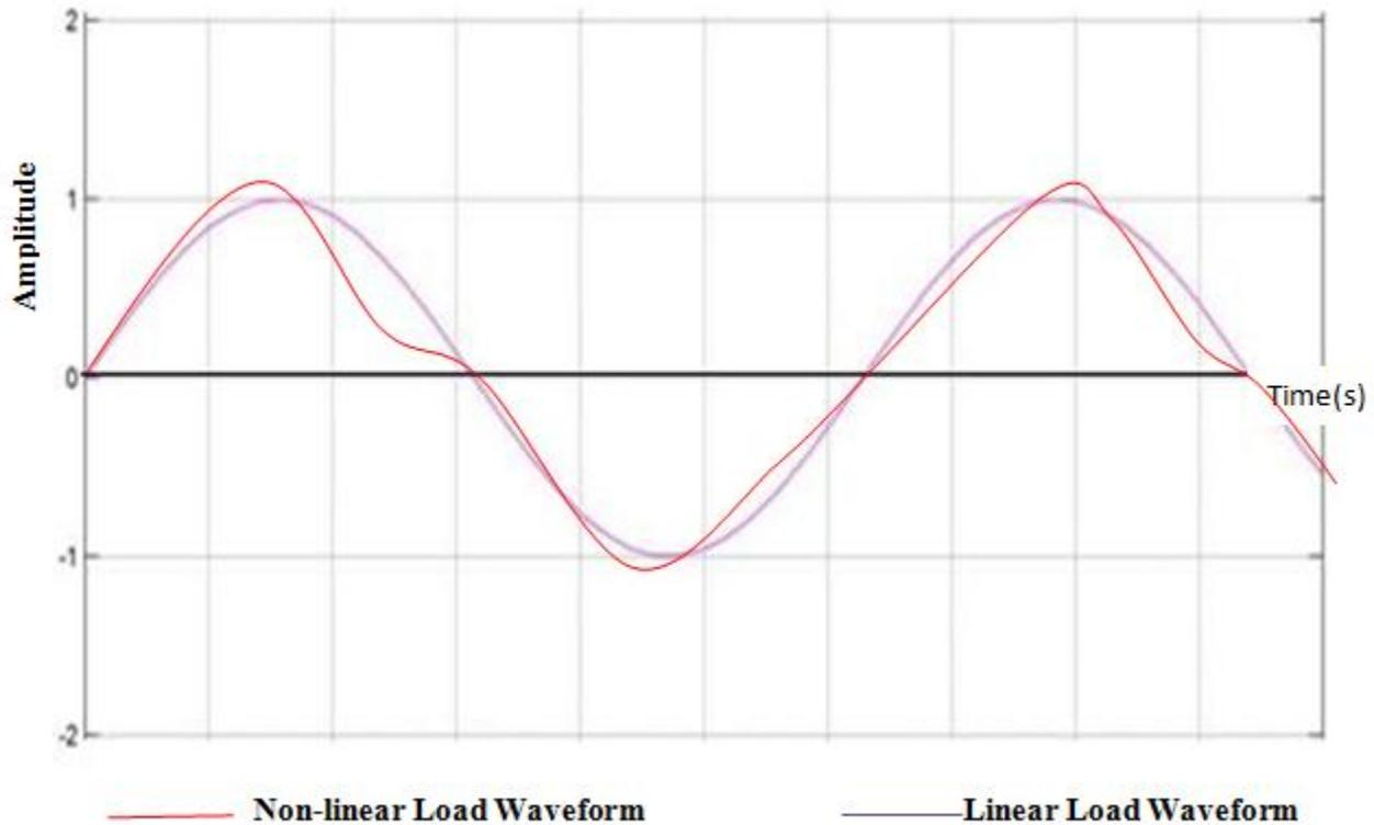
Fig. 1: Linear and Non-Linear Load Waveform
