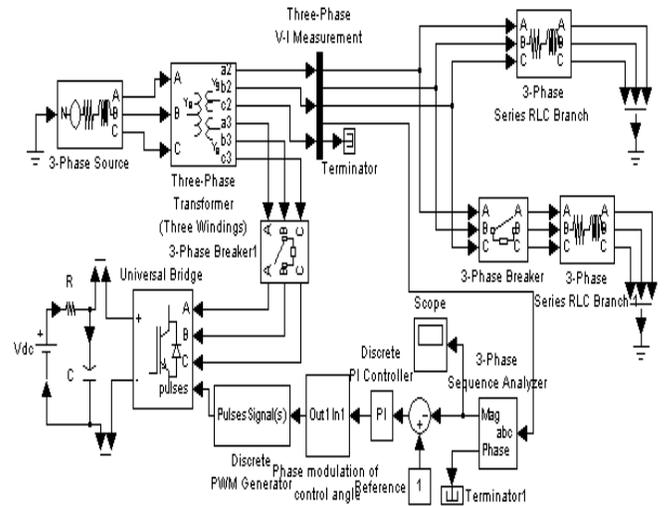
Fig 2: Simulink model for DSTATCOM
