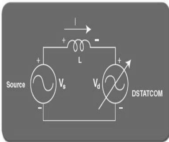
Fig.1. Test system for D-STATCOM
