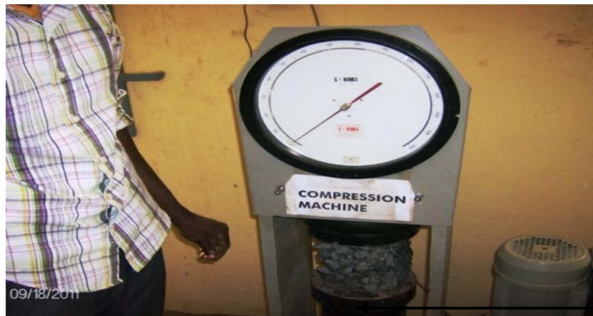
Figure 4: Compression Testing Machine (Controls Milano-Italy, range: 0 – 1500 kN)
