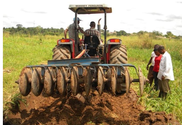
Plate 1.A photograph depicting tractor-dynamometer, implement mounted position during disc harrowing operations
