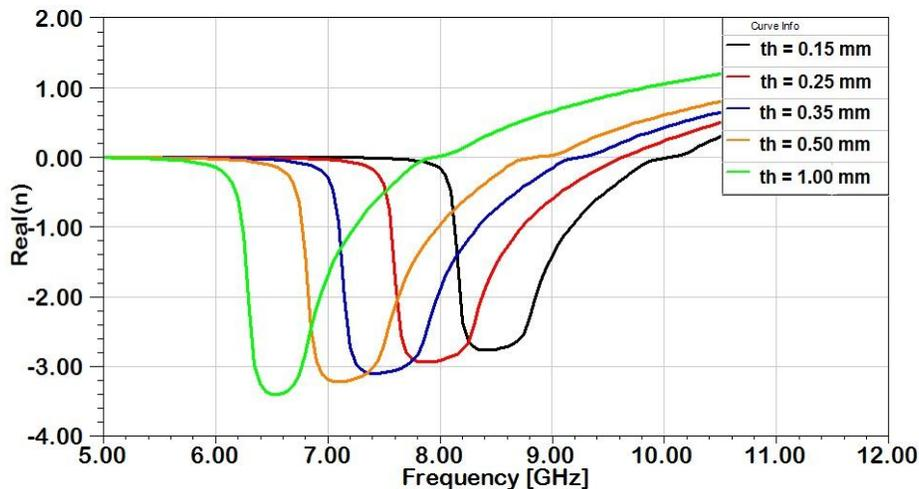
Figure 6:- Real part of refractive index  $n$  with different substrate thicknesses
