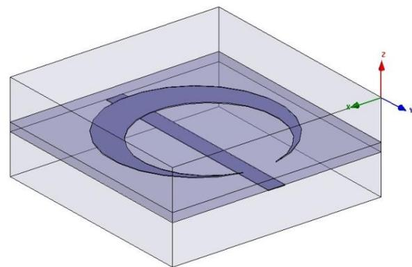
Figure 1:- The crescent shaped unit cell showing the excitation and propagation directions
