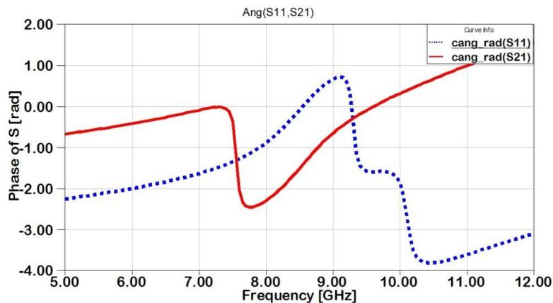
Figure 4:- Cumulative angle of  $S_{11}$  and  $S_{21}$
