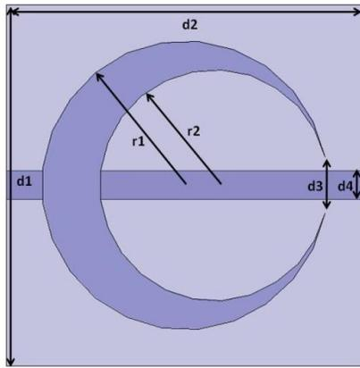
Figure 2:- The crescent shaped unit cell dimensions;  $d1 = d2 = 6 \text{ mm}$ ,  $d3 = 0.942 \text{ mm}$ ,  $d4 = 0.48 \text{ mm}$ ,  $r1 = 2.4 \text{ mm}$ ,  $r2 = 1.914 \text{ mm}$ .
