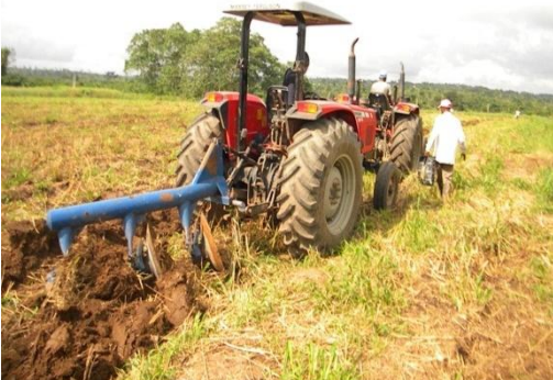
Plate 1. A photograph depicting tractor-dynamometer, implement mounted position during disc ploughing operations
