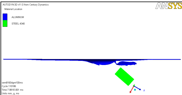
Fig.33 .Numerical impact pair model with 60° obliquity
