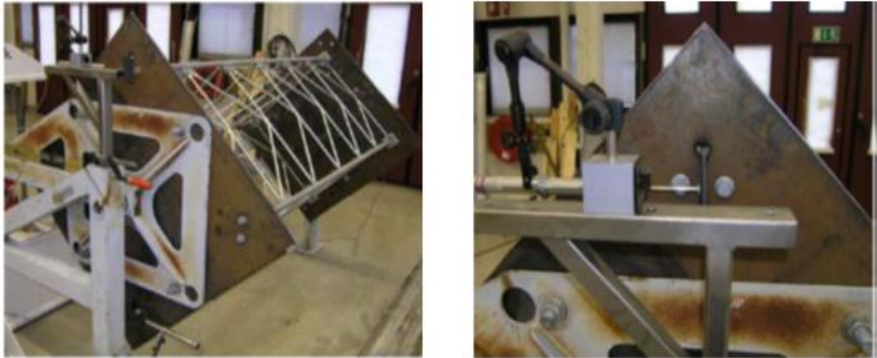
Figure 5: (a) Experimental setup: Flatpack section fixed to a rigid plate (b) Experimental setup: extensometer measuring the rotational displacement.
