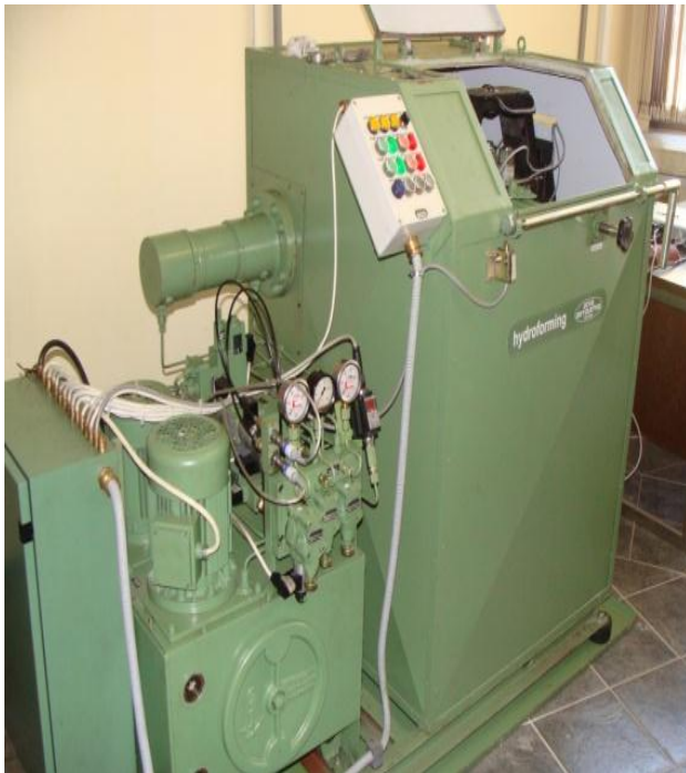
[Fig 3] Equipment for experimental analysis of tube hydroforming process
