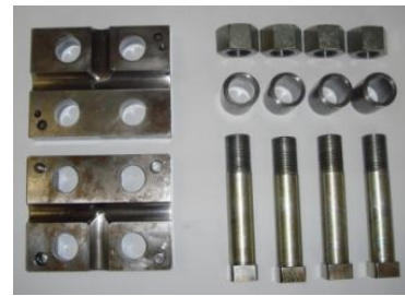
[Fig 4] T-shape tube hydroforming die
