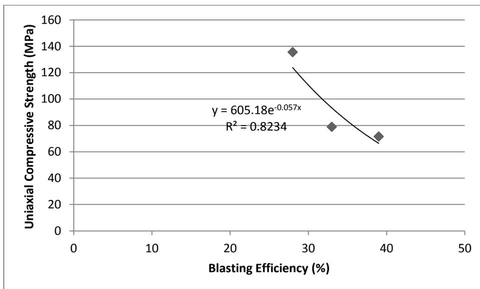
Figure 5: Correlation between Efficiency and Uniaxial Compressive Strength when Using ANFO
