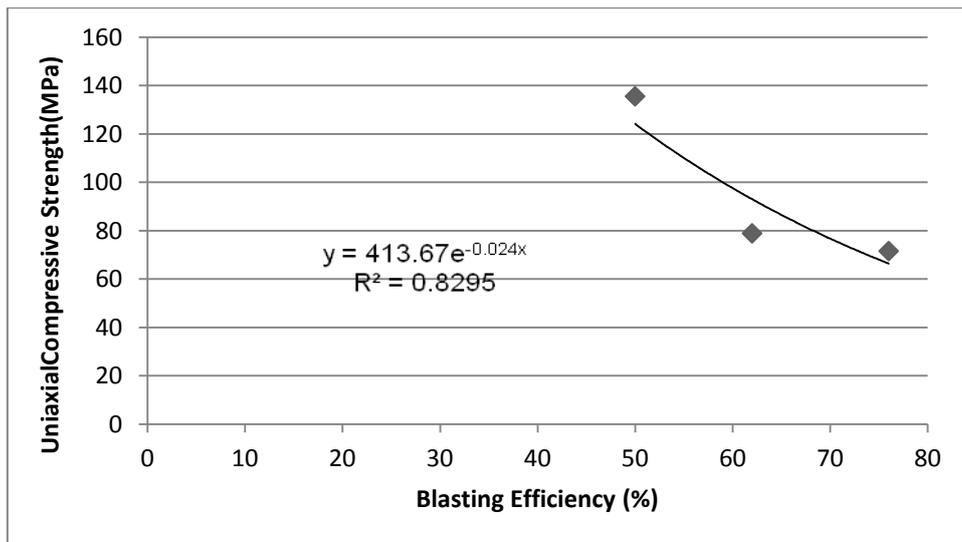
**Figure 3: Correlation between Efficiency and Uniaxial Compressive Strength when using Emulsion**
