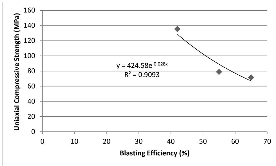
Figure 4: Correlation between Efficiency and Uniaxial Compressive Strength when Using Slurry
