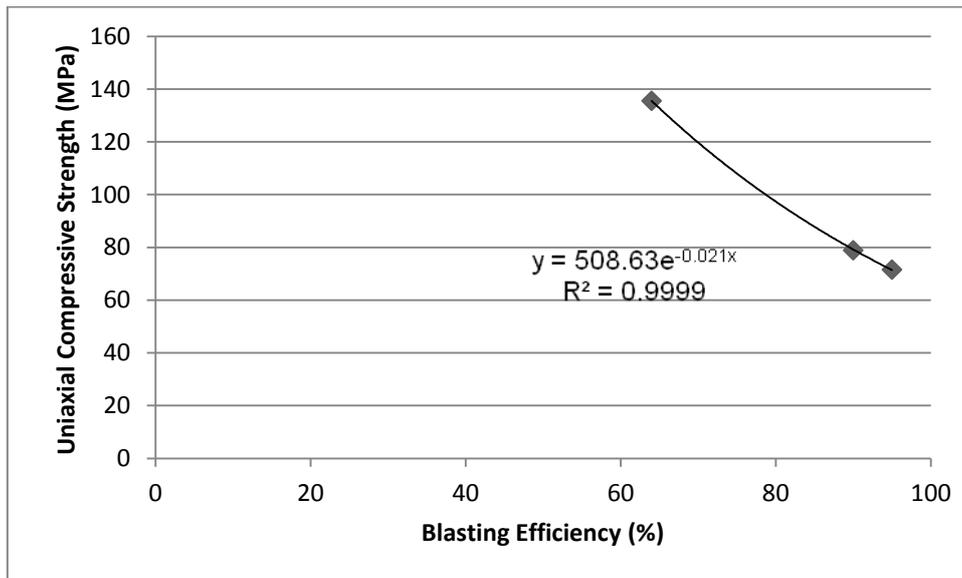
**Figure 2: Correlation between Efficiency and Uniaxial Compressive Strength when Using Special Gel**
