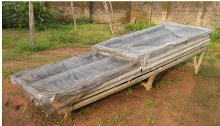
Figure 1: Solar dryer with metal plate solar thermal collector
