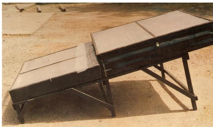
Figure 2: Solar dryer with wood solar thermal collector
