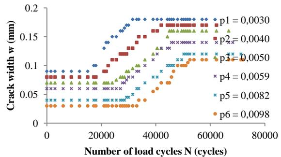
Fig. 4: Crack width versus number of load cycles for various reinforcement ratio
