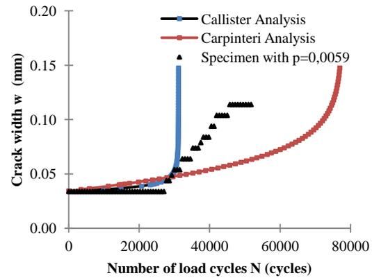
Fig. 3: Crack width at various analysis and experiment for precast deck slab
