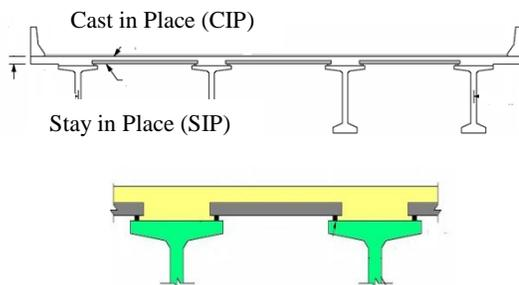
Fig. 1: Composite precast panel deck slab
