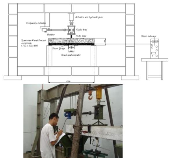
Fig. 2: Test setup and specimen geometry
