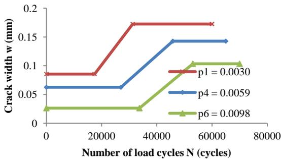
Fig. 6: Tri-linear model based on proposed formula
