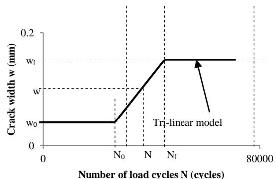
Fig. 5: Tri-linear model based on experimental analysis
