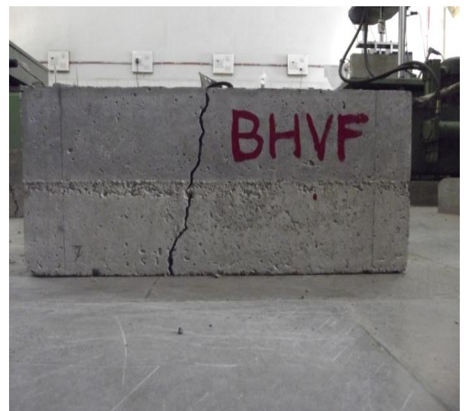
Figure 4: Typical failure pattern of composite beam under constant amplitude fatigue loading
