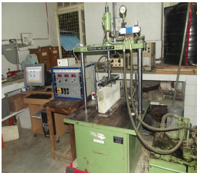
Figure 2: Flexural fatigue test setup
