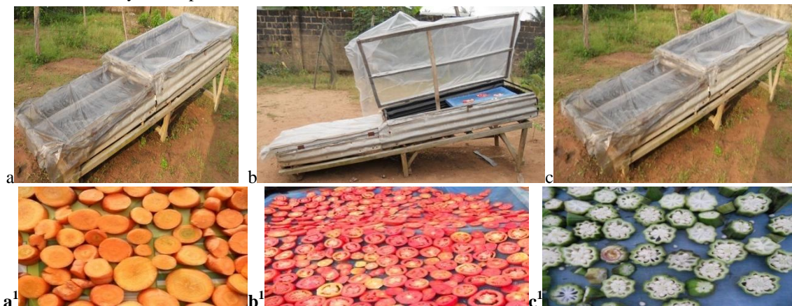
Figure 1: Three direct mode solar vegetable dryers, ( a, b and c are solar dryers for carrot, tomato and okra respectively. While a 1 , b 1 and c 1 are carrot, tomato and okra respectively)
