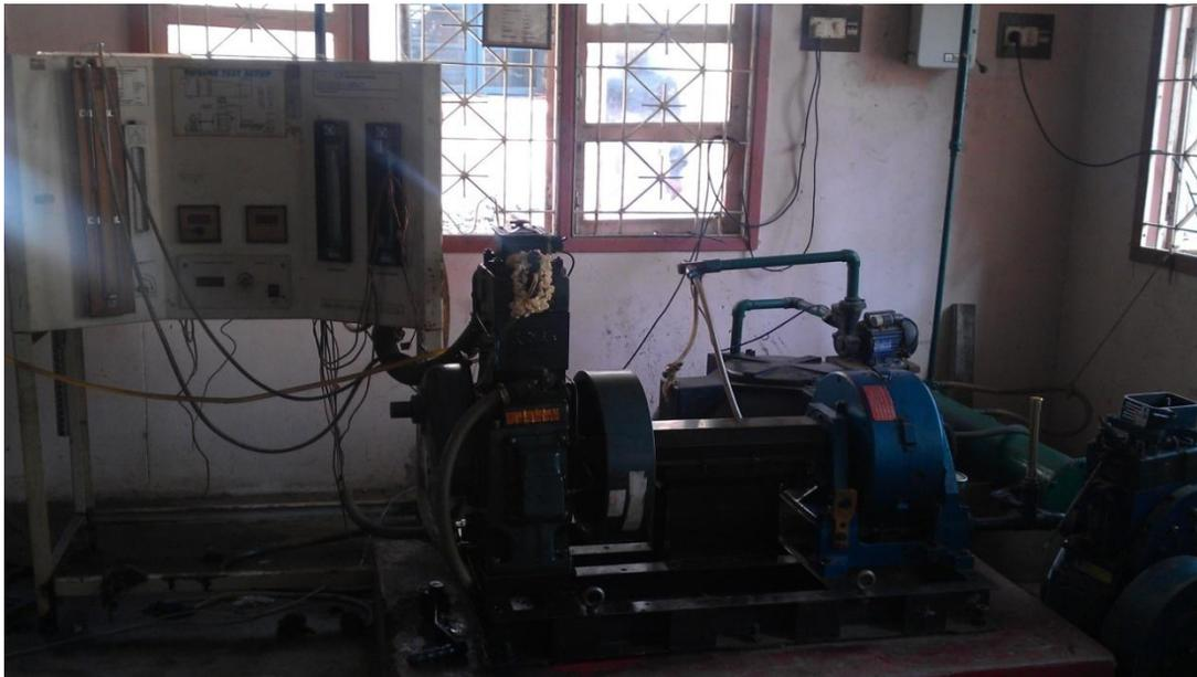
Fig. 3 Photographic view of engine setup
