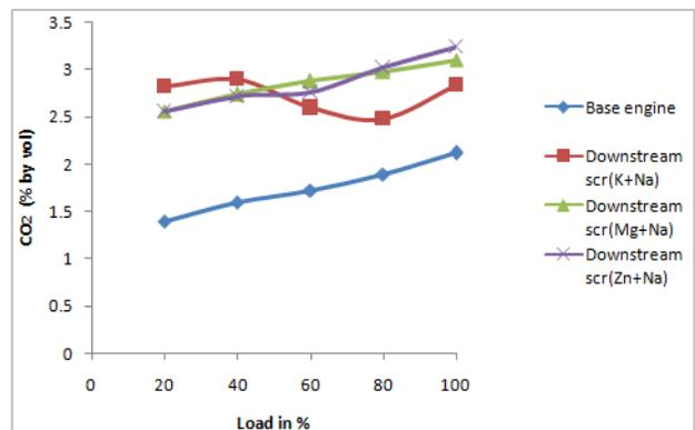
Fig.11 Effects of engine load in percentage on CO<sub>2</sub> emissions
