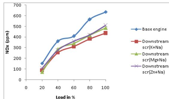
Fig.8 Effects of engine load in percentage on NOx emissions
