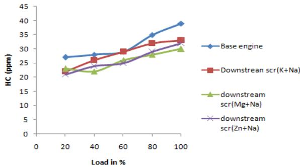
Fig.9 Effects of engine load in percentage on HC emissions
