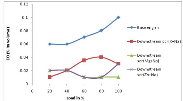
Fig.10 Effects of engine load in percentage on CO emissions
