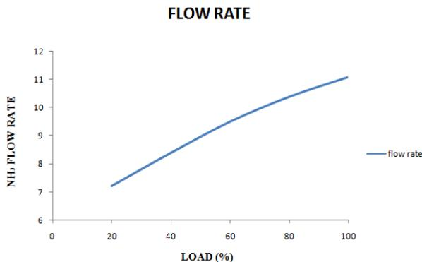
Fig.1 Mass flow rate of Ammonia Vs Load
