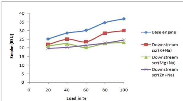
Fig.12 Effects of engine load in percentage with Smoke emission
