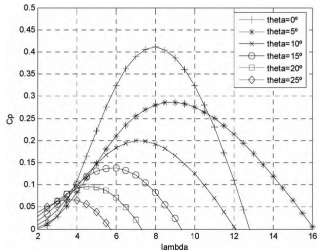
Figure 1: The graph of Coefficient of power ( $C_p$ ) versus Tip-speed ratio ( $\lambda$ )
