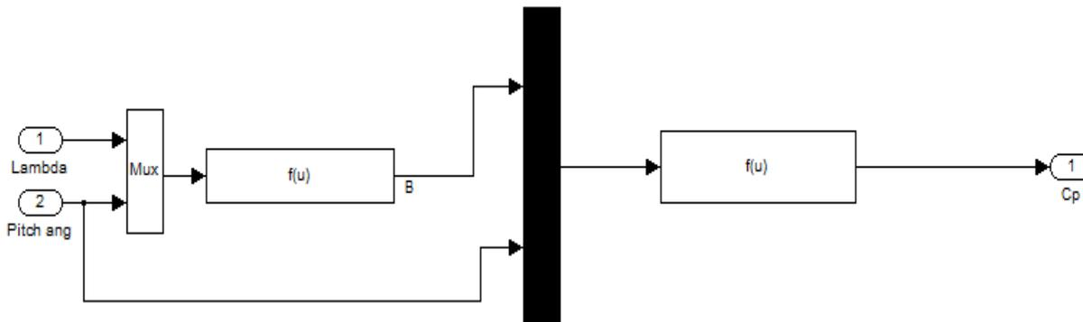
Figure 5: Coefficient of power, Cp calculation Model
