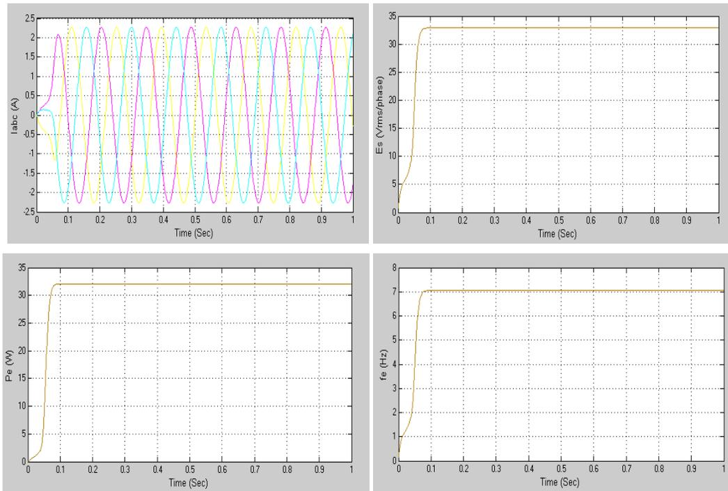
**Figure 10: Graph of the Three Phase Current, The Voltage, The Electromagnetic Power and The Electrical frequency at a Wind speed of 3m/s**
