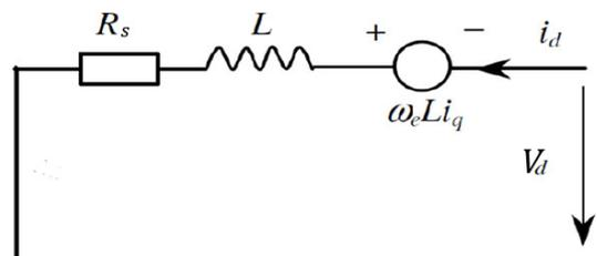
Figure 2: d-axis equivalent circuit
