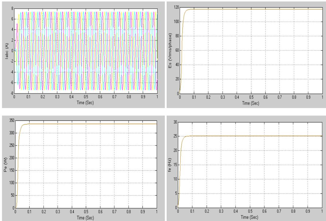
**Figure 11: Graph of the Three Phase Current, The Voltage, The Electromagnetic Power and The Electrical frequency at a Wind speed of 6m/s**
