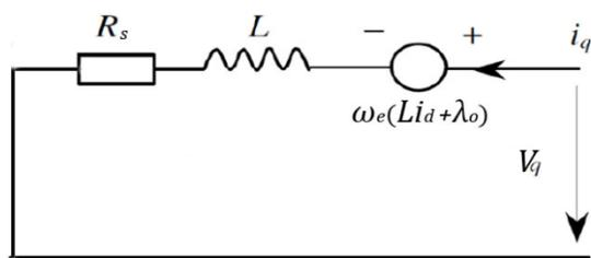
Figure 3: q-axis equivalent circuit
