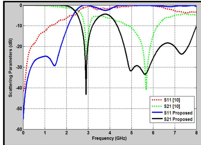
Figure (5) The scattering parameters of the proposed filter compared to the double equilateral U-shaped DGS low pass filter presented in [10]
