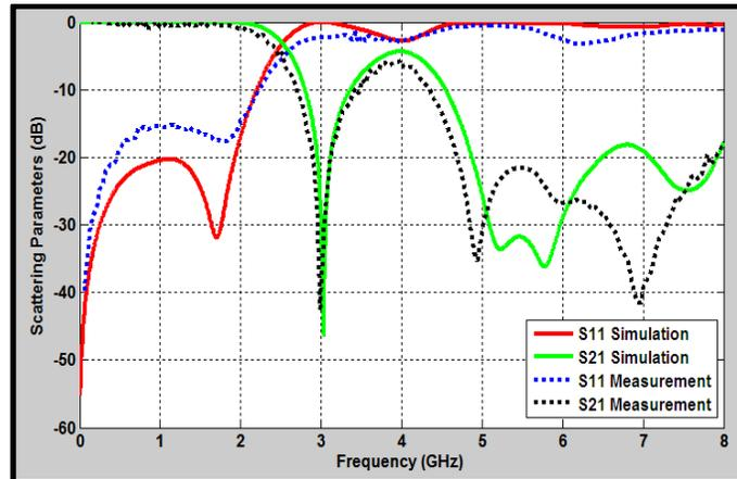
Figure (8) The scattering parameters of the proposed low pass filter obtained using the CST ready-made simulator compared to the experimental measurement results
