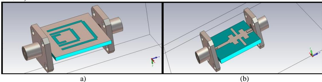
Figure (3) - (a) back view, and (b) front view of the simulated CST design of the proposed low pass filter
