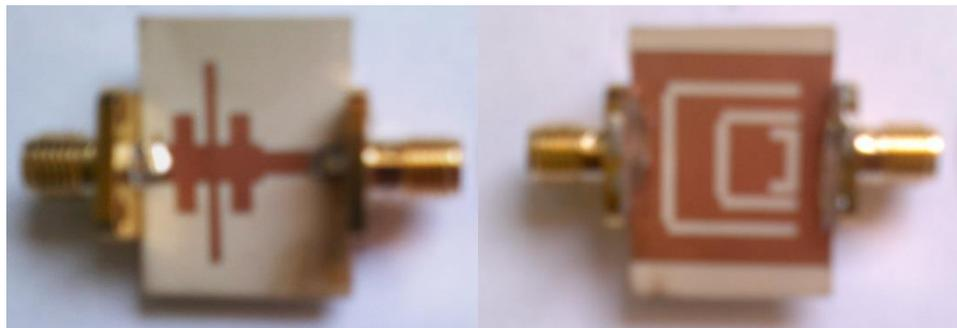
Figure (6) The picture of the fabricated filter on Rogers RO3003 substrate
