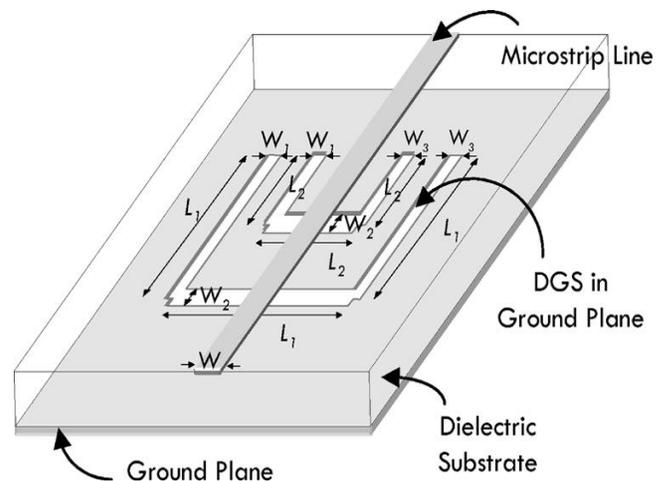
Figure (1) Three-dimensional view of the DGS unit [10]
