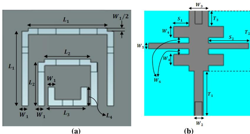
Figure (4) Description of the (a) DGS unit and (b) the transmission line dimensions
