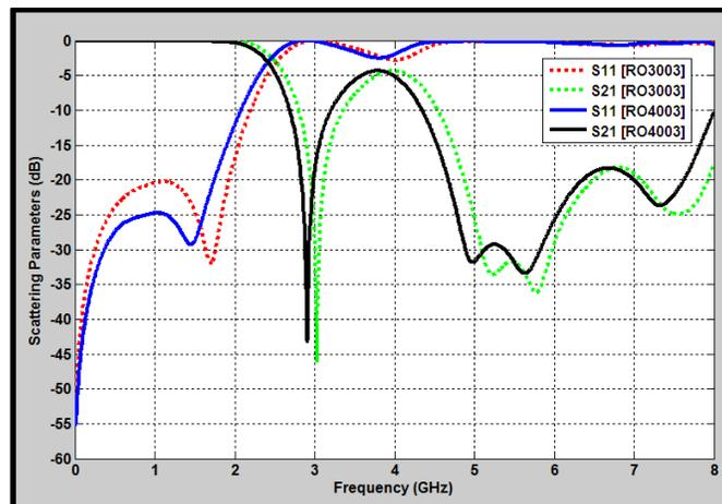
Figure (7) Frequency shift occurred in the simulated scattering parameters using Rogers RO4003 versus Rogers RO3003 substrates
