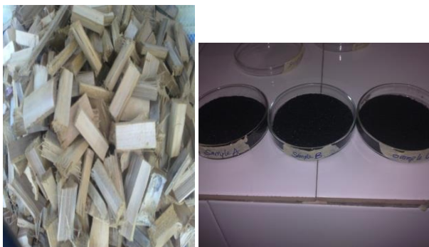
Fig 1. Waste bamboo before and after carbonization and activation
