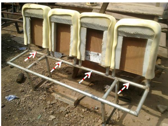
Fig. 1: Locally Fabricated Vehicle Seat during Construction (Arrows Pointing To Base Rear Connecting Member)
