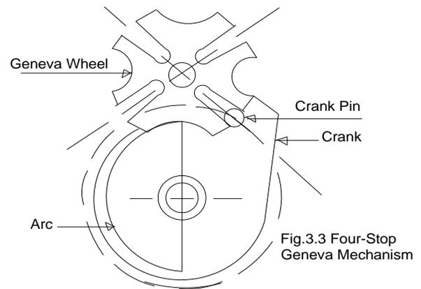
Fig.3.3 Four-Stop Geneva Mechanism
