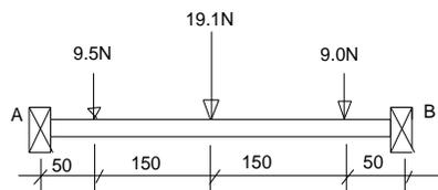
Fig.3.2 Main Shaft Loading
