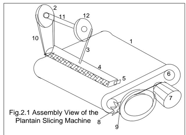
Fig.2.1 Assembly View of the Plantain Slicing Machine
