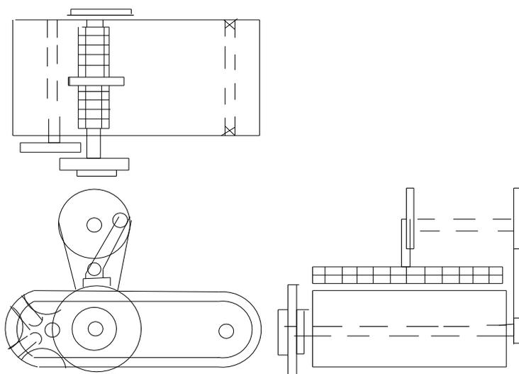
Fig.2.2 Orthographic View of the Plantain Slicing Machine
