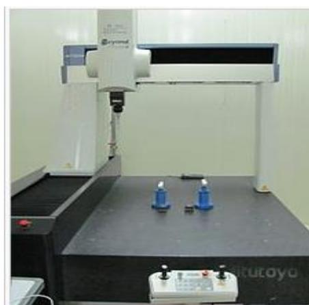
Figure 3: Coordinate Measuring Machine
