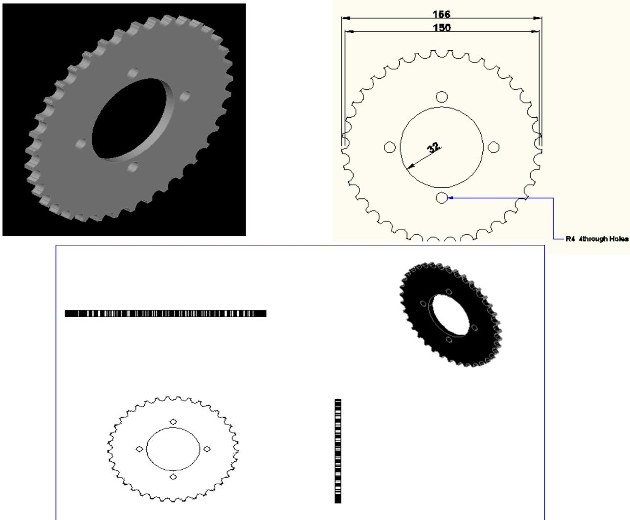
Figure 5: Sprocket 3D standard view drawn with AutoCAD
