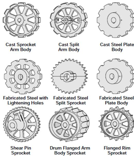
Figure 1: Sprocket Styles
