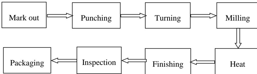
**Figure 6: Manufacturing layout of a CY80 Motorcycle Rear Sprocket**
