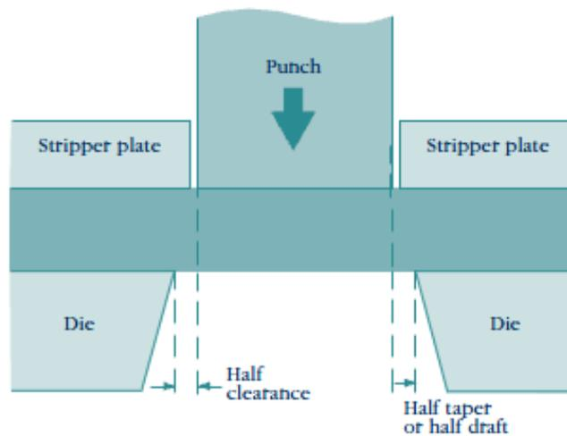
**Figure 7: Features of a Punch**
