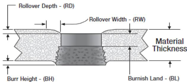
Figure 9: Anatomy of a punched Hole
