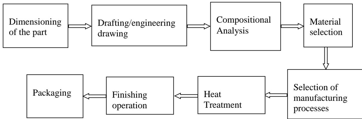
Figure 2: Generic Layer out of RE Operations for sprocket Production
