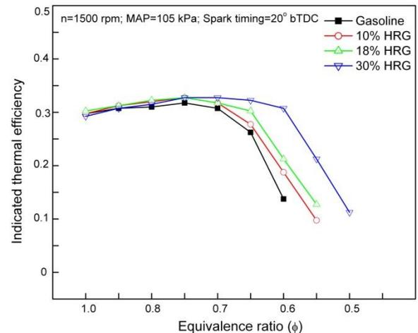
Fig.8 Indicated thermal efficiency Vs Equivalence ratio
