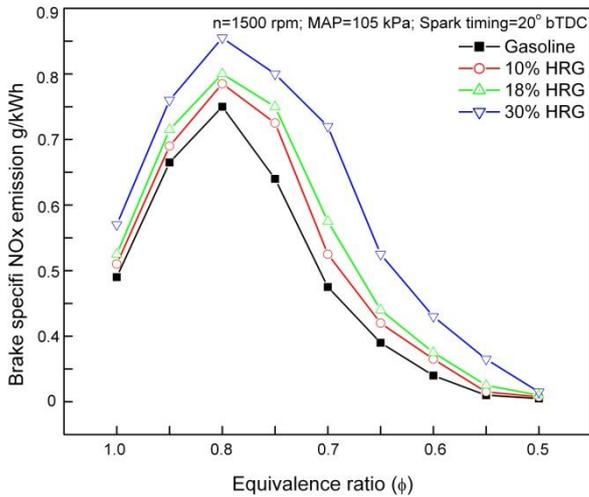
Fig.5 Brake specific NOx Vs Equivalence ratio
