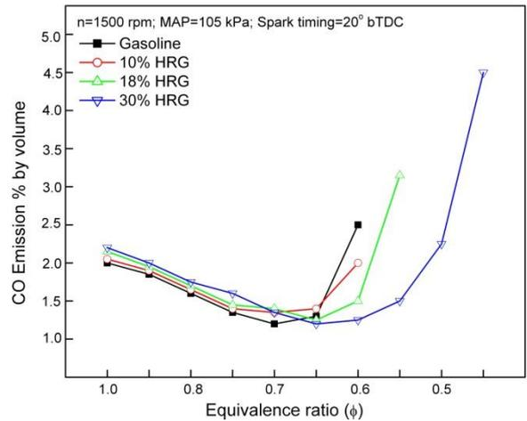
Fig.7 Brake specific CO Vs Equivalence ratio
