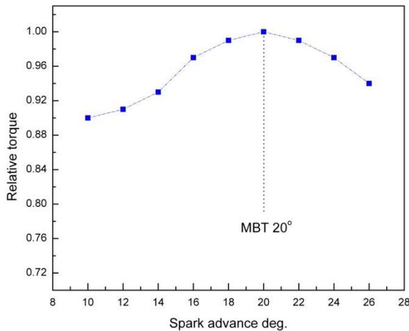
Fig.2 Relative torque Vs spark advance
