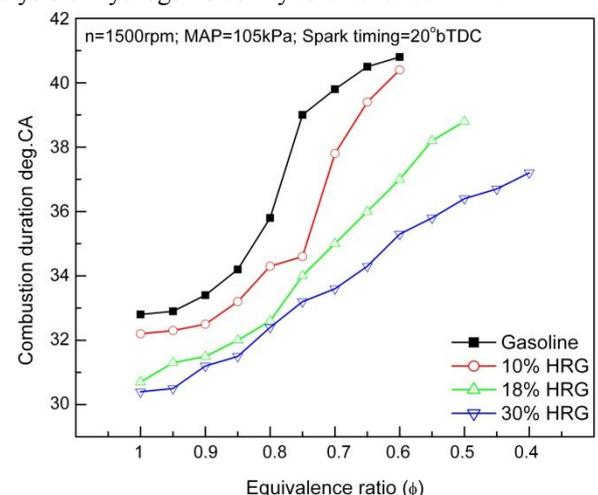
Fig.4 Combustion duration Vs Equivalence ratio
