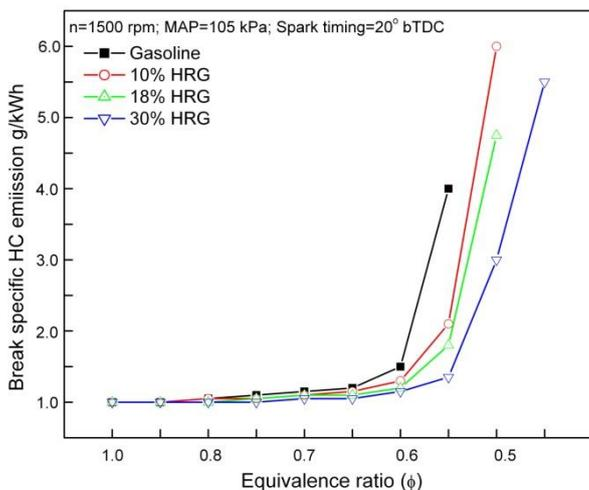
Fig.6 Brake specific HC Vs Equivalence ratio
