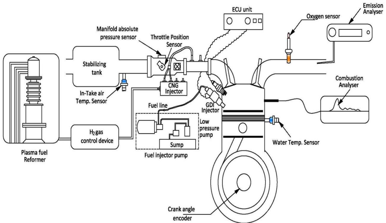
Fig.1 Experimental configuration of Lean Burn Engine
