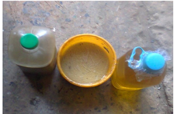
Plate 4: Sample of crude oil, sludge and refined groundnut oil (from left to right)
