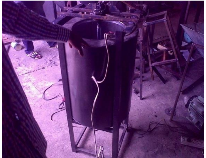
Plate 2: Fabrication in progress Stirrer, heater terminals and pulley.
