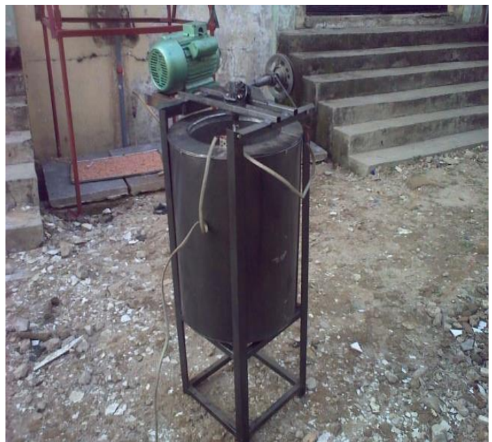
Plate 3: The first unit of the clarifying system after fabrication
